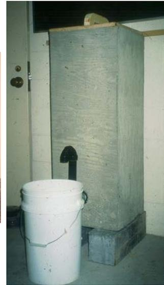
Wood mold Nicaragua 1994. Wood mold proved not durable and was replaced by the more durable steel mold.
