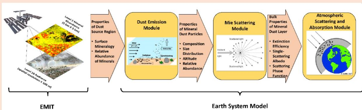
Figure 14.17 Data is collected from sensor mounted on the ISS and provided to earth system models <https://earth.jpl.nasa.gov/emit/mission/about/> and <https://earth.jpl.nasa.gov/emit/documents/3/> .
