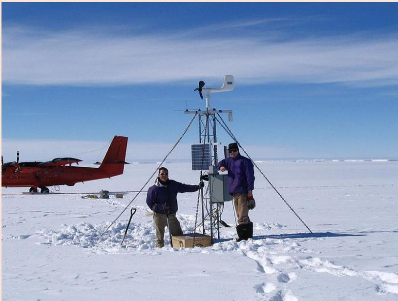
Figure 14.7 Antarctic automatic weather station – part of the automatic weather stations project AWS in Antarctica [https://en.wikipedia.org/wiki/Automatic\\_weather\\_station](https://en.wikipedia.org/wiki/Automatic_weather_station) .
