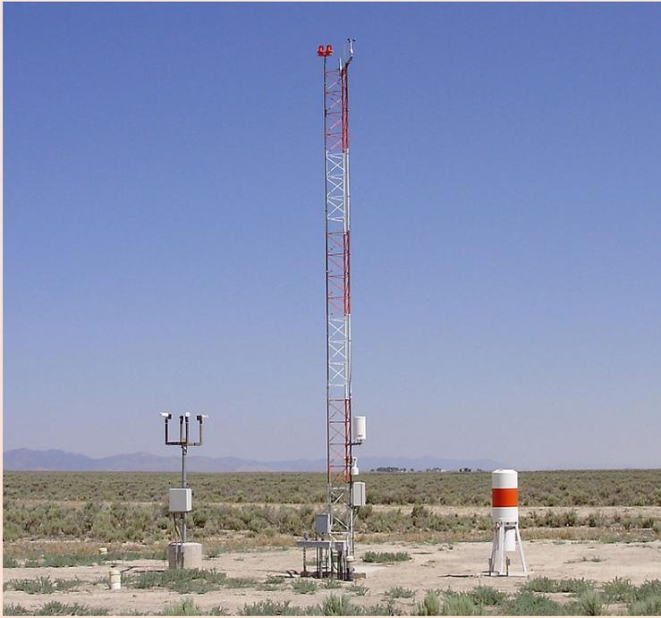
Figure 14.8 Commercial automatic weather observation station AWOS.
