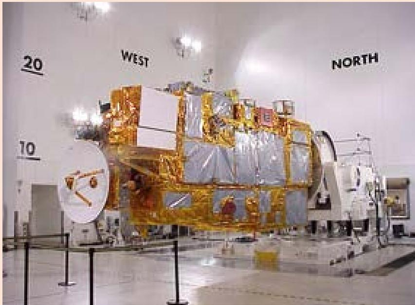
Figure 14.21 NASA Terra satellite <https://terra.nasa.gov/about> . Carries five instruments, Advanced Spaceborne Thermal Emission and Reflection Radiometer (ASTER), Clouds and Earth's Radiant Energy System (CERES), Multi-angle Imagine Spectroradiometer (MISR), Measurements of Pollution in the Troposphere (MOPITT) and Moderate Resolution Imaging Spectroradiometer (MODIS).
