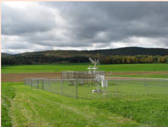
Figure 14.3 Modern surface weather station, U.S. Climate Reference Network Station, Ithaca, New York.
