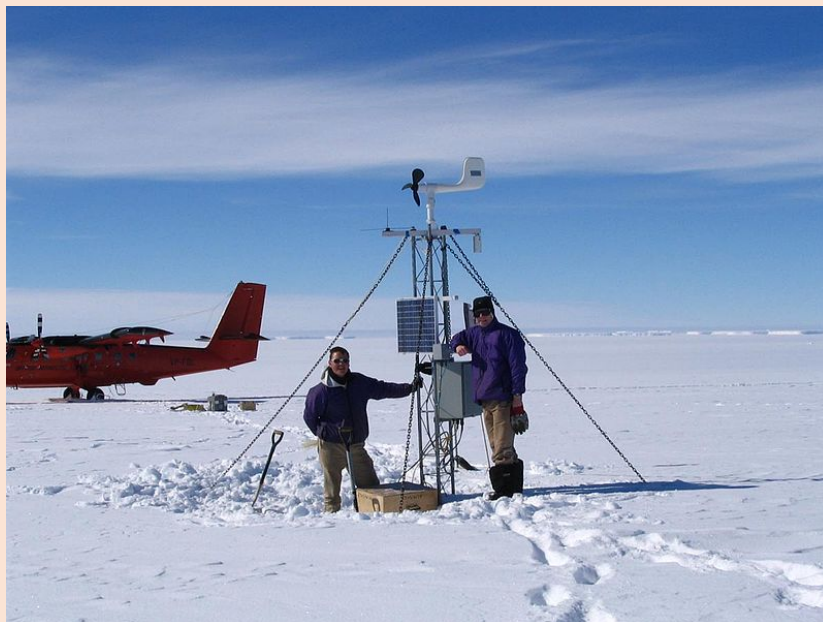
Figure 14.7 Antarctic automatic weather station – part of the automatic weather stations project AWS in Antarctica.
