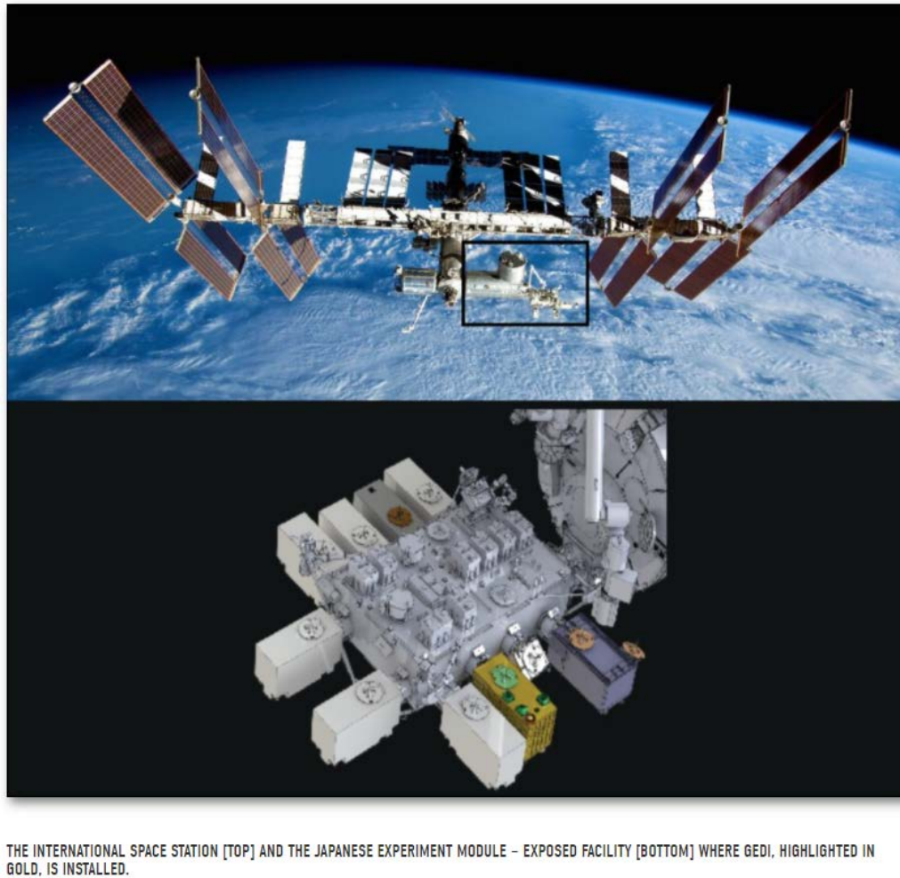
Figure 17.14 GEDI, shown in gold, as mounted on the International Space Station.
