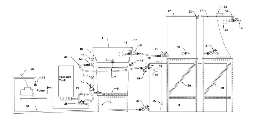
Figure 1 - Automated System Layout - Aeration System and Additional Head Tank
