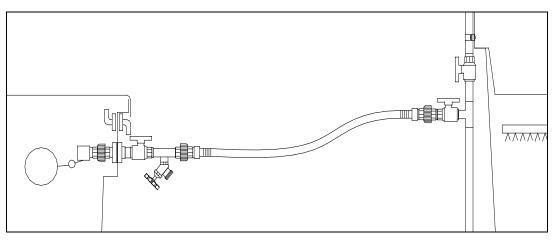
BioSand Filter and GA Carbon Water Filter Coupler.
