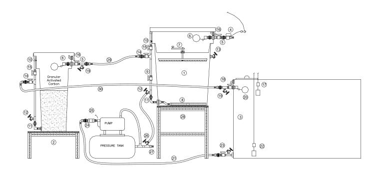
Figure 1 - Automated System Layout - BioSand Filter and GA Carbon Water Filter
