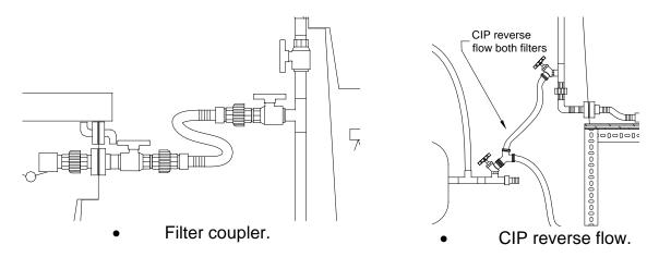
**Step 4.** Locate the CIP reverse flow assembly. Connect the wye fitting to the CIP reverse flow faucet. Connect the hose from the wye to the lower valve on each filter standpipe. **Step 5.** Return to the manual and continue with the installation.
