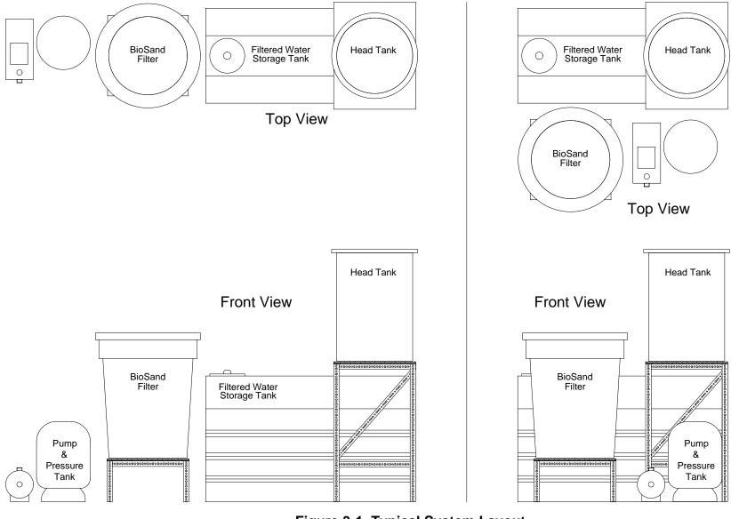
Figure 3-1 Typical System Layout
