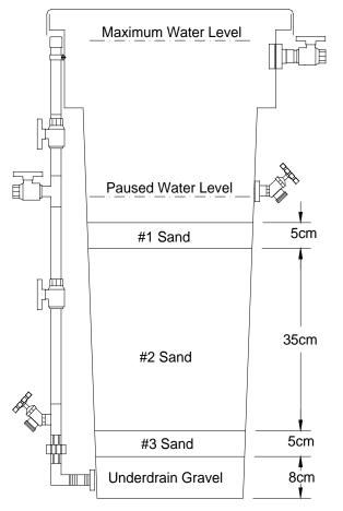
Figure 4-1 Filter Media and Filter Water Levels
