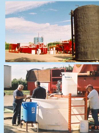
Setting Up Field Test Reactors for 4 Cubic Meter Tests on Flowback Water in Brooks, Alberta
