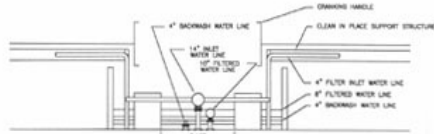
SECTION A - A PIPE ARRANGEMENT NOT TO SCALE
