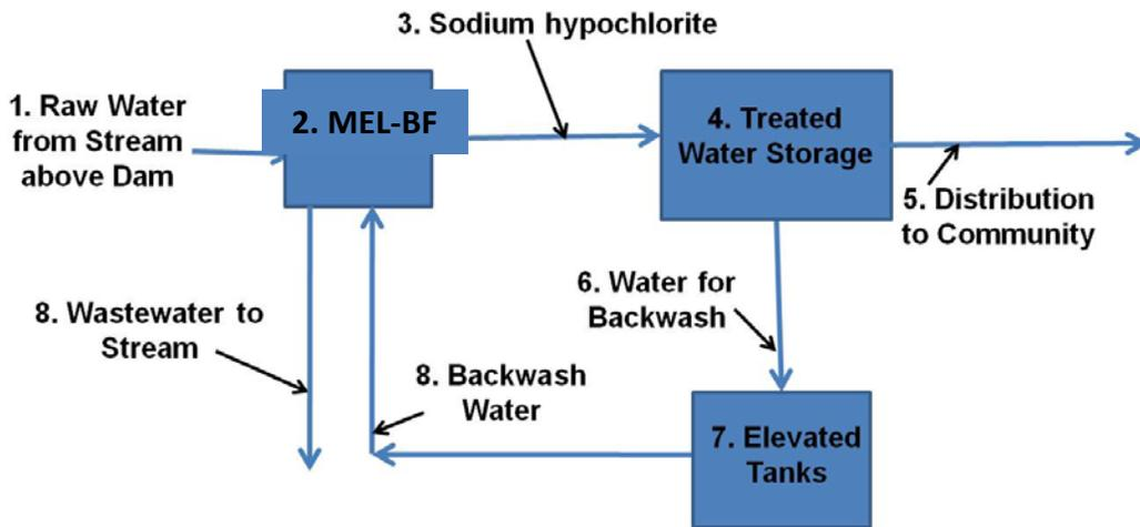
Figure 3. Process flow diagram for the Punta Huina water treatment plant.
