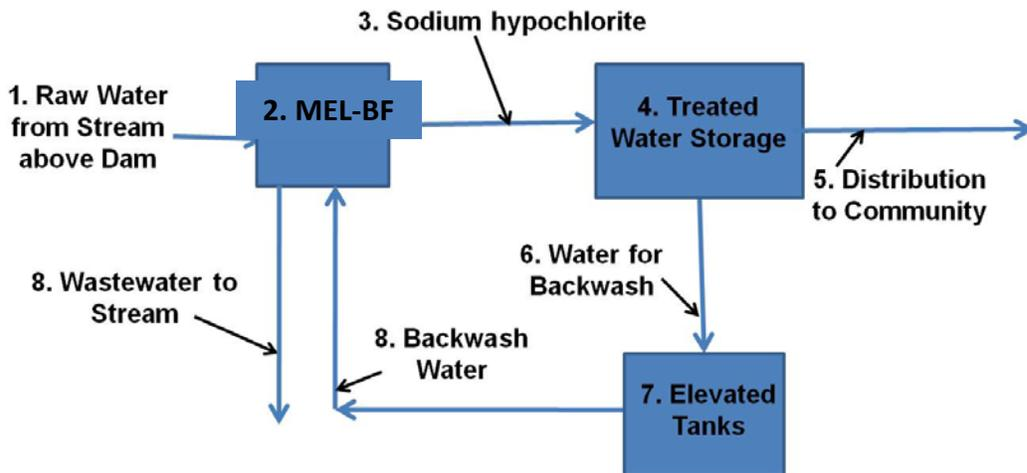
Figure 3. Process flow diagram for the Punta Huina water treatment plant.
