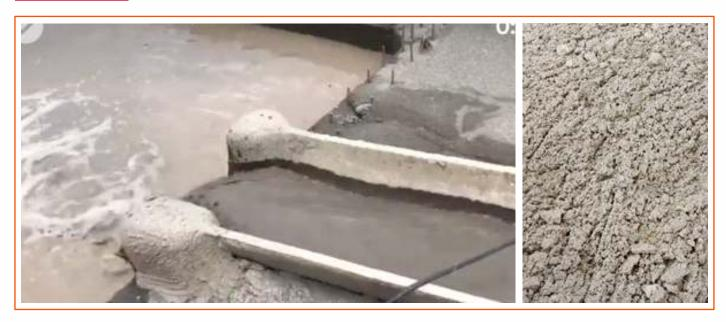
Most dangerous and notorious product generated from the process of washing is sludge. It is not processable. The material contains up to 40% moisture. It cannot be dried because it forms pebble like particles which would need grinding after drying. It cannot be used as road filler because the density keeps varying a lot and is completely unpredictable in compaction. Also dangerous because it can turn into quick sand during heavy rains.
