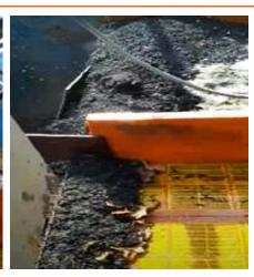
Washed Sand is the purest form of sand. It is a very good product for making wall plasters. The sand will contain almost 0% slit, free of -50 & -75 Microns product. This sand can be packed in bags and sold over the counter as premium plaster sand. The entire city of Bangalore uses this sand for their plastering need. There is negligible sale of ready plaster and the masons prefer only this sand.
