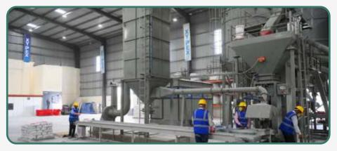
Apollo dry mortar plant basically consists of a drying systems, loading system, conveying & weighing system, highly accurate weighing system to mix sand, cement and additives in required proportion where it finally gets the exact composition of the required mortar. Once it is prepared, dry mortar is available for bagging & ready to be transported to market. Apollo manufactures 5 TPH, 10 TPH, 15 TPH, 20 TPH, 25 TPH, & 30 TPH capacity plants.
