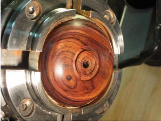
15. O-ring Groove & Bearing Seat Completed
