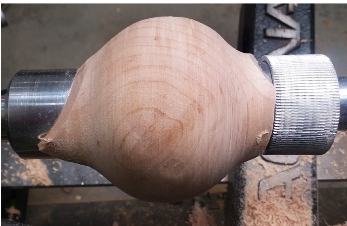
5 — Remove the wood to the outline of the sphere.
