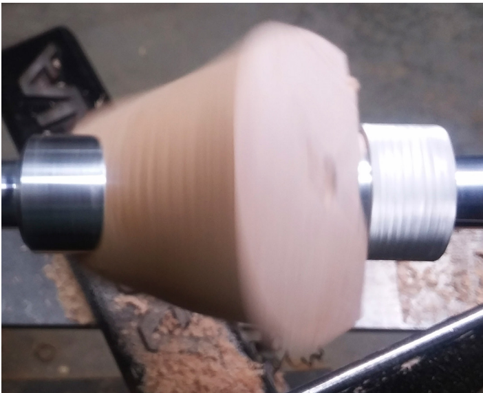
4 — As your cylinder turns, you'll have air gaps on both sides, you'll see the outline of the sphere in the center. My rpm was set at 700.
