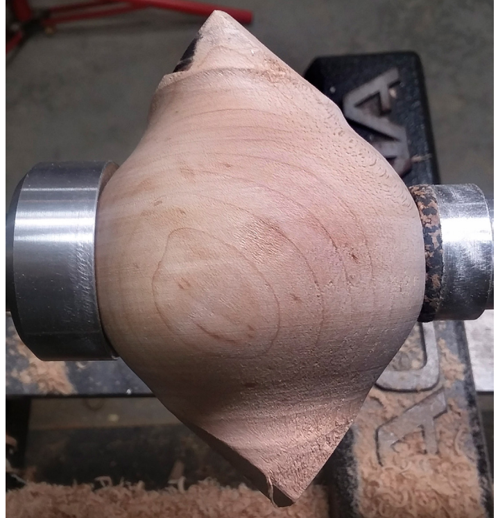
6 — After removing the first set of jigs, rotate the wood 90 degrees and insert it between the next set of jigs. These are cone shaped. The left side is solid metal and the right side has a cork top material, if you look close on the shaft you'll see a small pin in a slot. This is spring loaded to the proper tension when collapsed.
