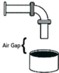
*Air gap: Must be twice the size of water supply outlet, but never less than 1 inch*
