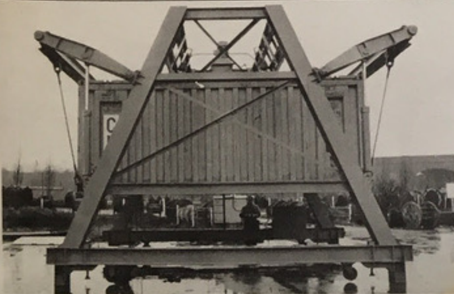
This mobile container handling unit weighs 7½ tons and is capable of lifting all containers to ISO specifications.
