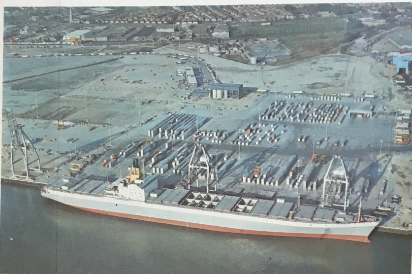
The 73,596-tonne "Benalder", seen here at Southampton, completed her maiden voyage—via Hamburg, Rotterdam, Southampton, Singapore, Hong Kong and Japan—before the New Year. Her British-made GEC turbine engines can develop a maximum of 88,000 shp giving a service speed of 26 knots and a maximum of over 30 knots.
