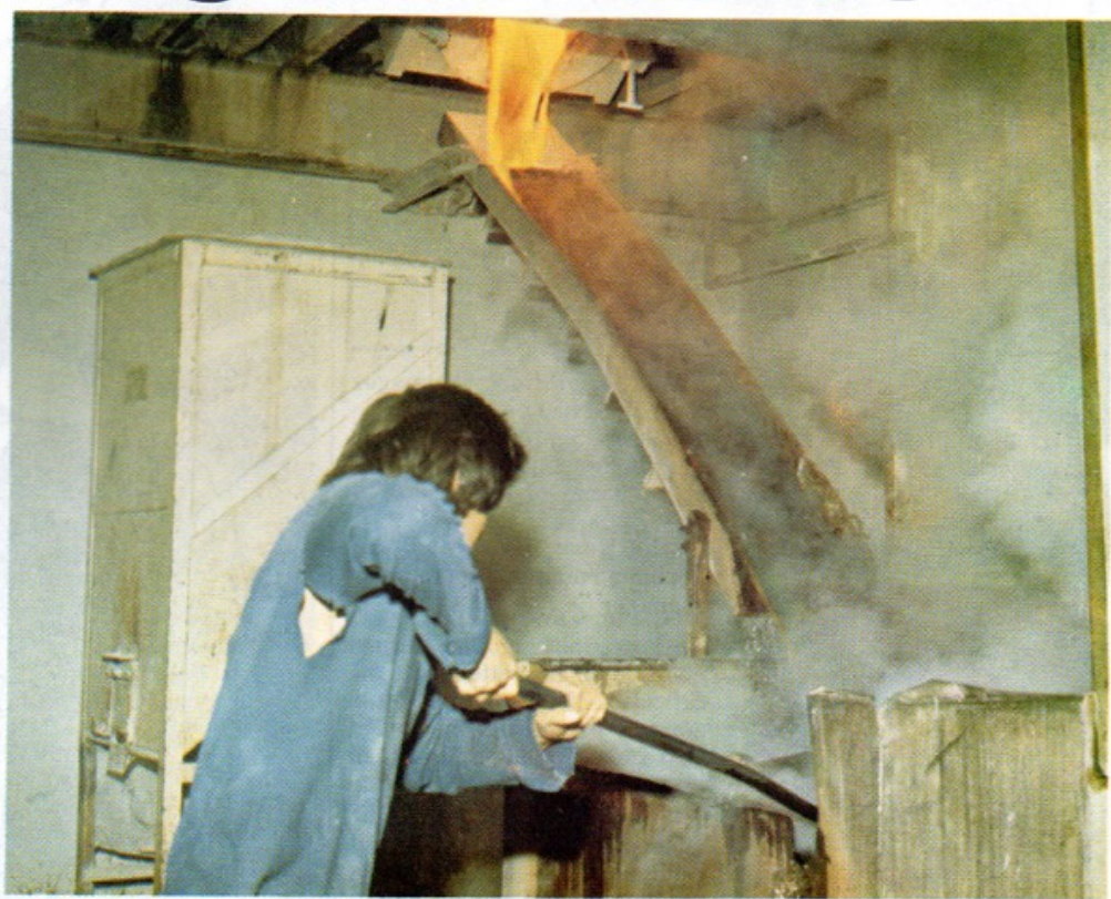
A worker helps keep the Zircon liquid from solidifying at Podmore and Sons' ceramics plant at Stoke-on-Trent during the refining process.
