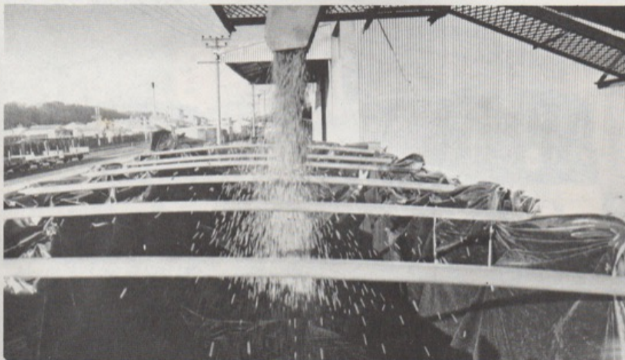
Maple peas being loaded in bulk by a mechanical conveyor belt at Christchurch for shipment by ACTA to Johnston and Jeff of Hull.
