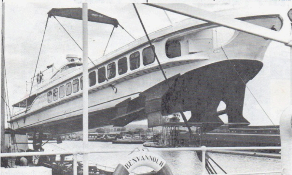
Shortly before starting its voyage to Manila, a Raketa hydrofoil is loaded on board Ben Line's vessel "Benvannoch" in London. Much of the ancillary equipment on this Russian-built craft is of British manufacture. It has a cruising speed of 40 mph and will be used as a ferry.
