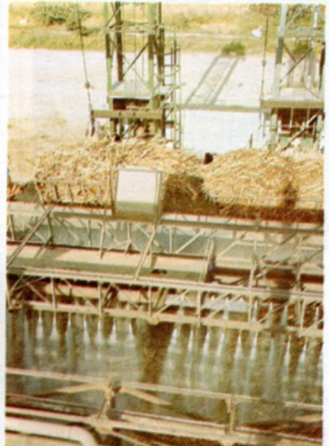
Cut cane arrives at the factory and is washed down in the first stage of the process.
