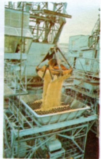
After taking a giant bite, the jaws open and the sugar is dropped into a hopper and onto the conveyor belt.
