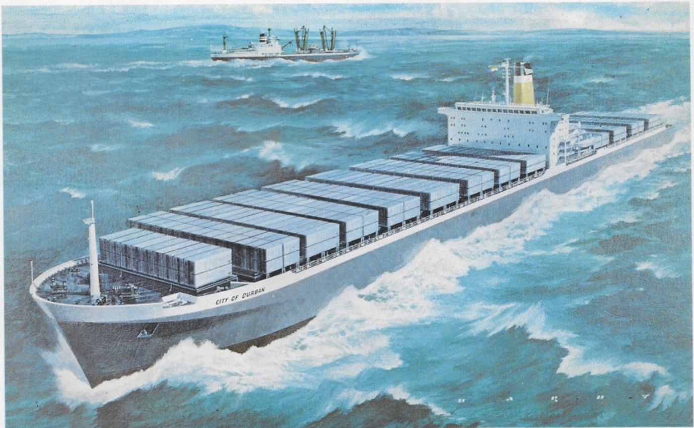
EHCL's fully cellular containership, "City of Durban" which is now under construction, and when completed later this year will carry some 2,500 twenty-foot equivalent units and will provide regular container service to South Africa.
