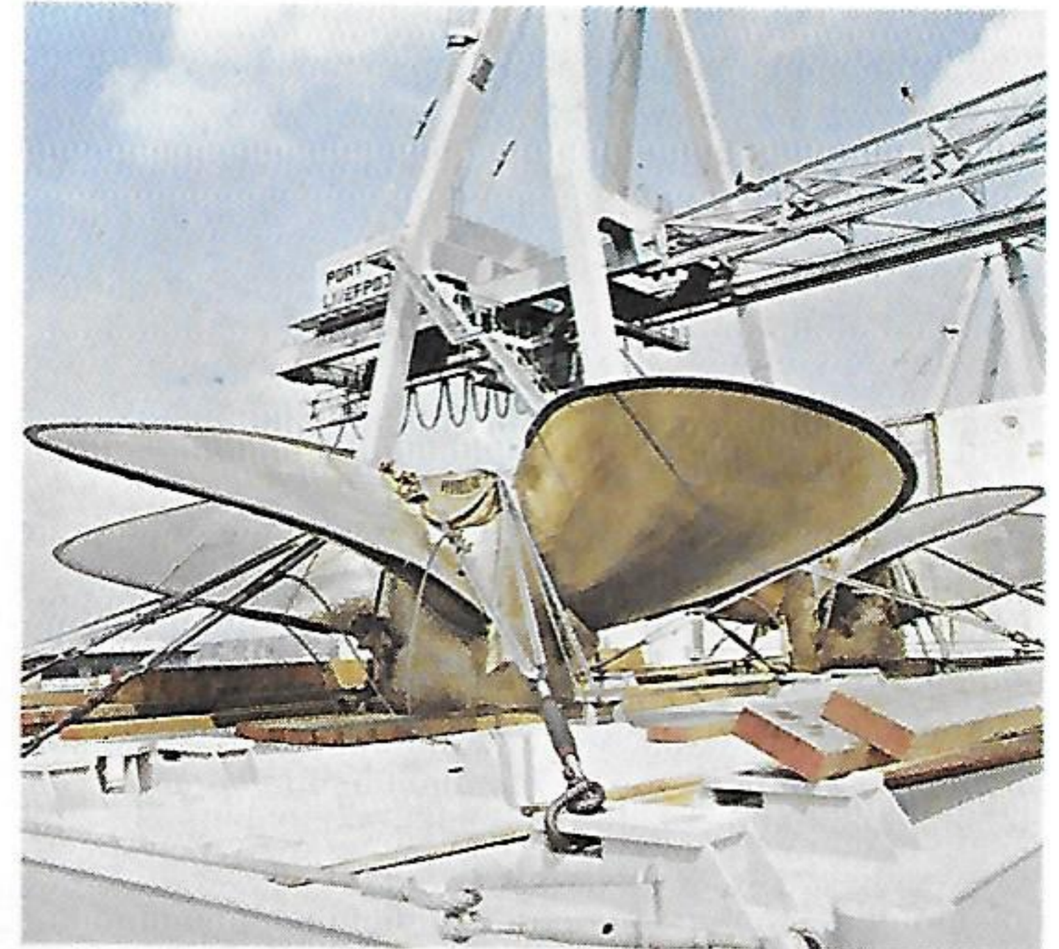
Two spare propellers for "ACT 7's" sister ship, "Australian Venture", carried on the forward deck.
