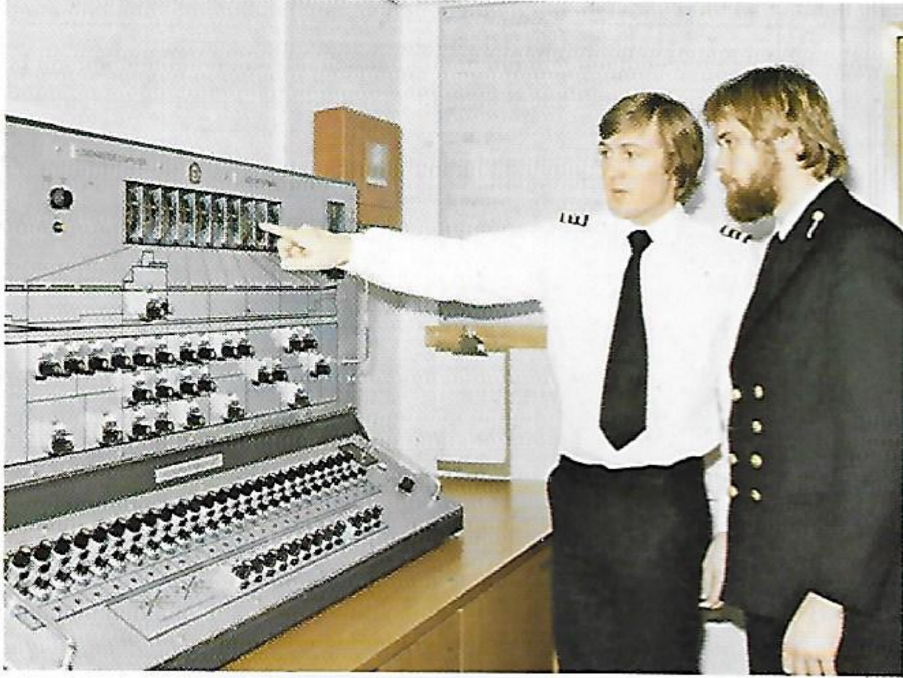
Computing the stability of the ship to ensure that the cargo weight is equally distributed along the length of the vessel is First Officer David Miller (left) shown explaining the process to Deck Cadet Michael Samus.
