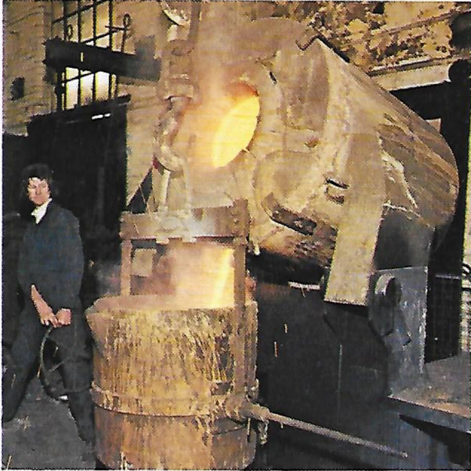
The metal for casting the bells, which has been heated to a tremendously high temperature, is poured from the furnace into the ladle.
