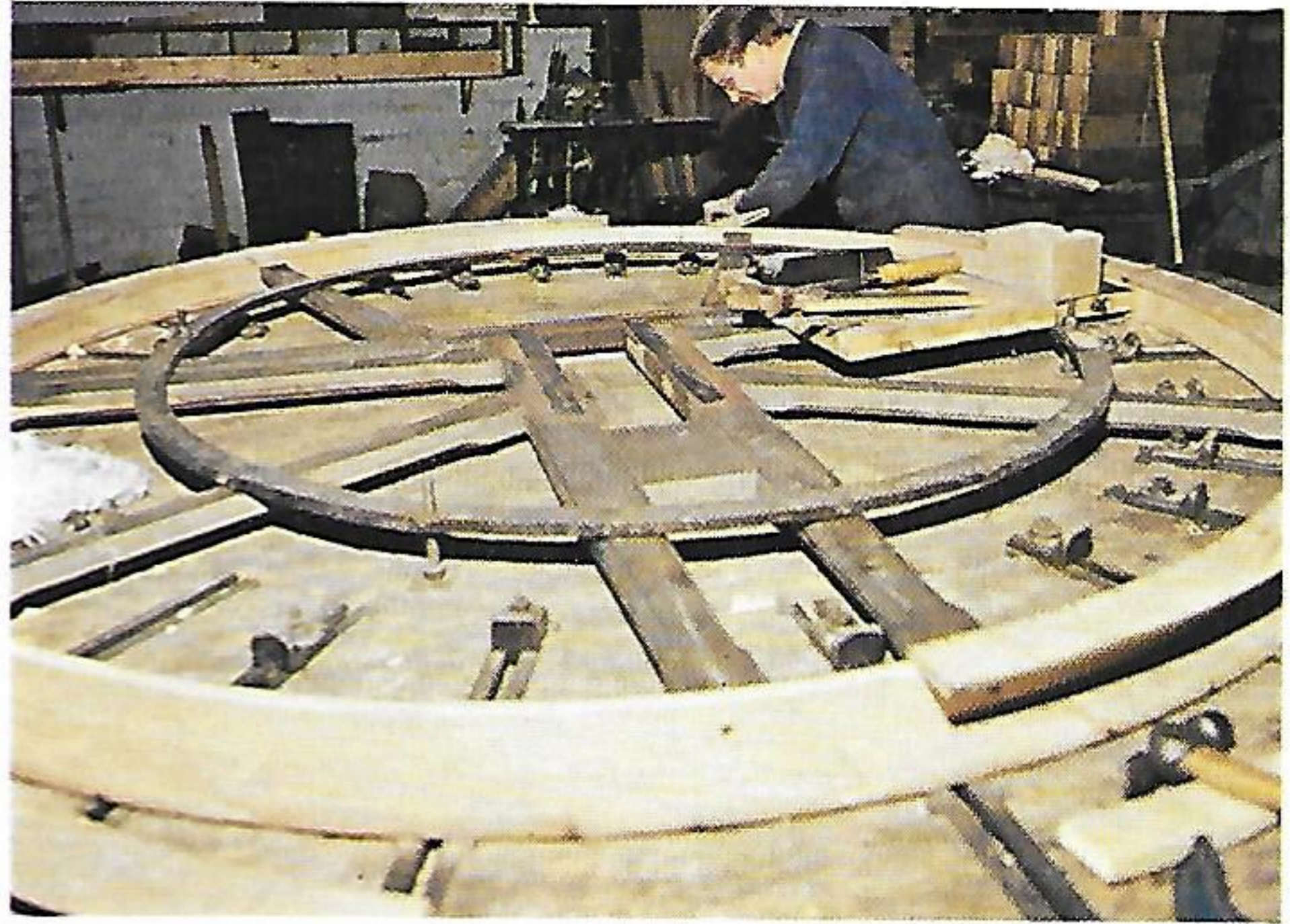
A bell wheel is being made in the carpenter's shop which will be fitted to the beam on which the bell is hung, allowing the bellringer to operate it more easily because of the large size of the wheel.
