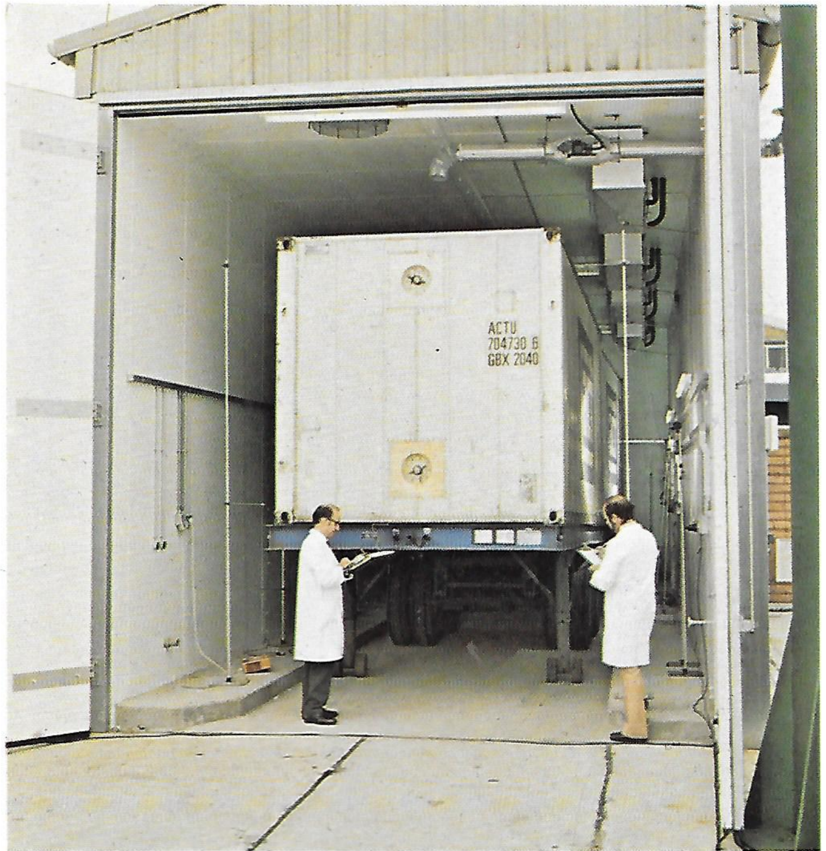
One of the newest additions to SRCRA's facilities in this test chamber capable of taking a 40' refrigerated container or two 20' boxes.
