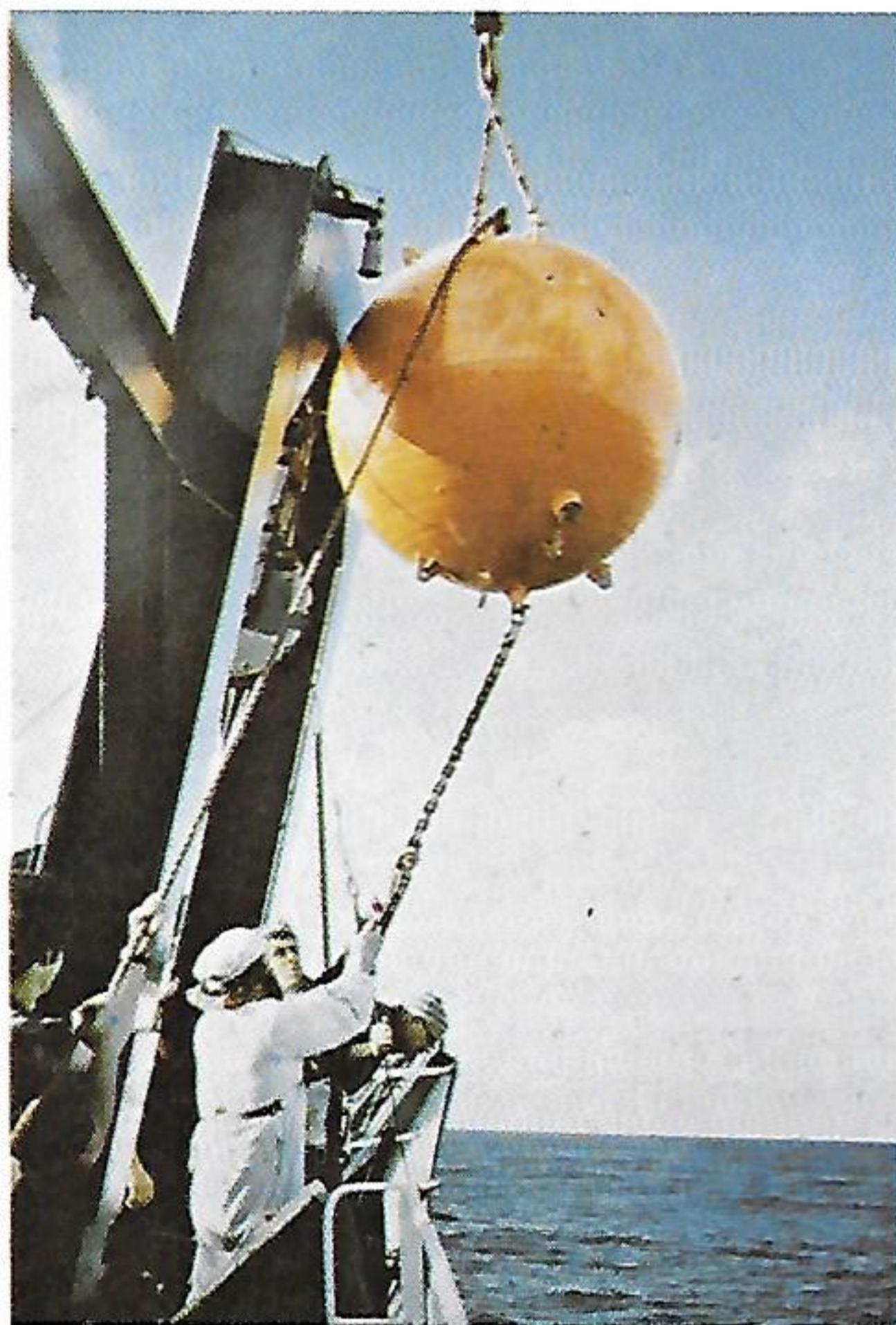
A subsurface buoy ready to be lowered from the "Discovery". It is attached to underwater equipment and will eventually be used to bring the equipment back to the surface.
