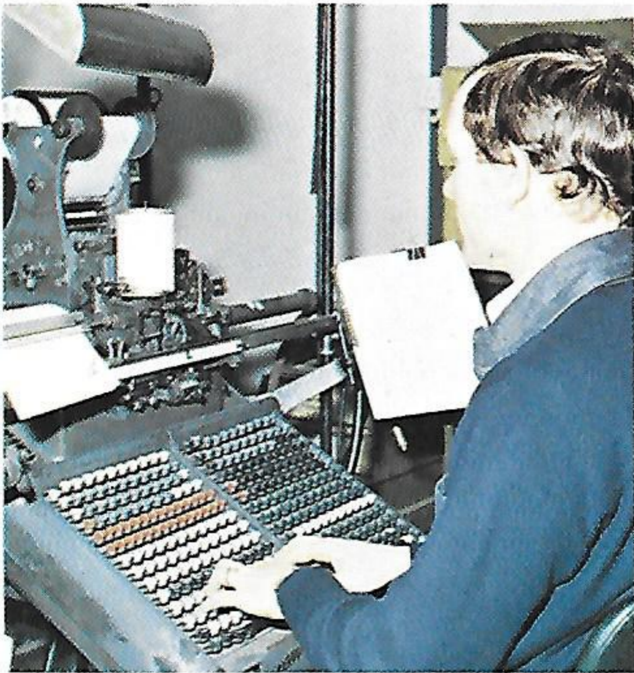
It all begins with typesetting. Very little is set by hand today and linotype and hot metal appear to be slowly giving way to photo composition and other modern methods.
