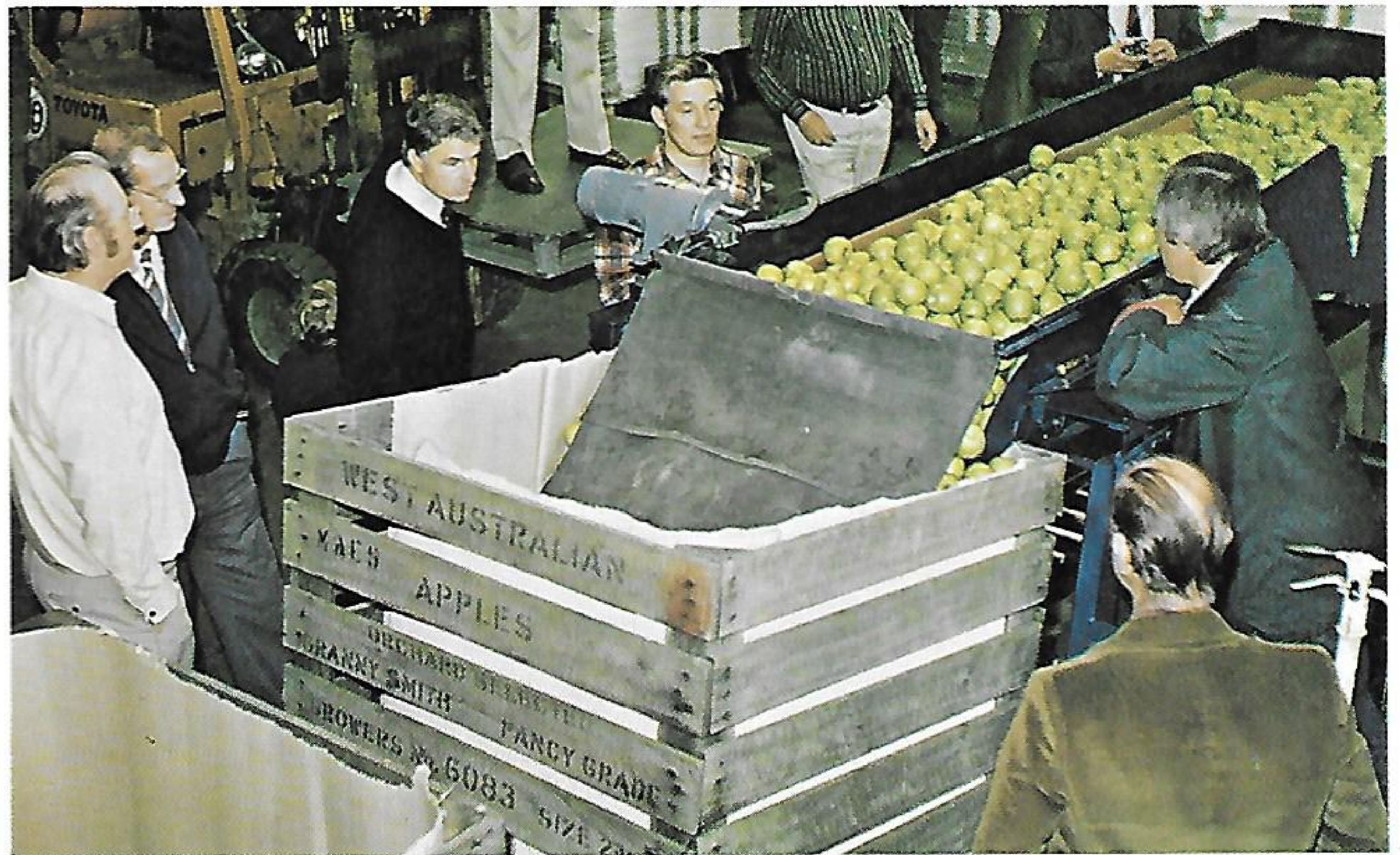
The apples are discharged into 29-bushel bins at the rate of 2½ minutes per bin.
