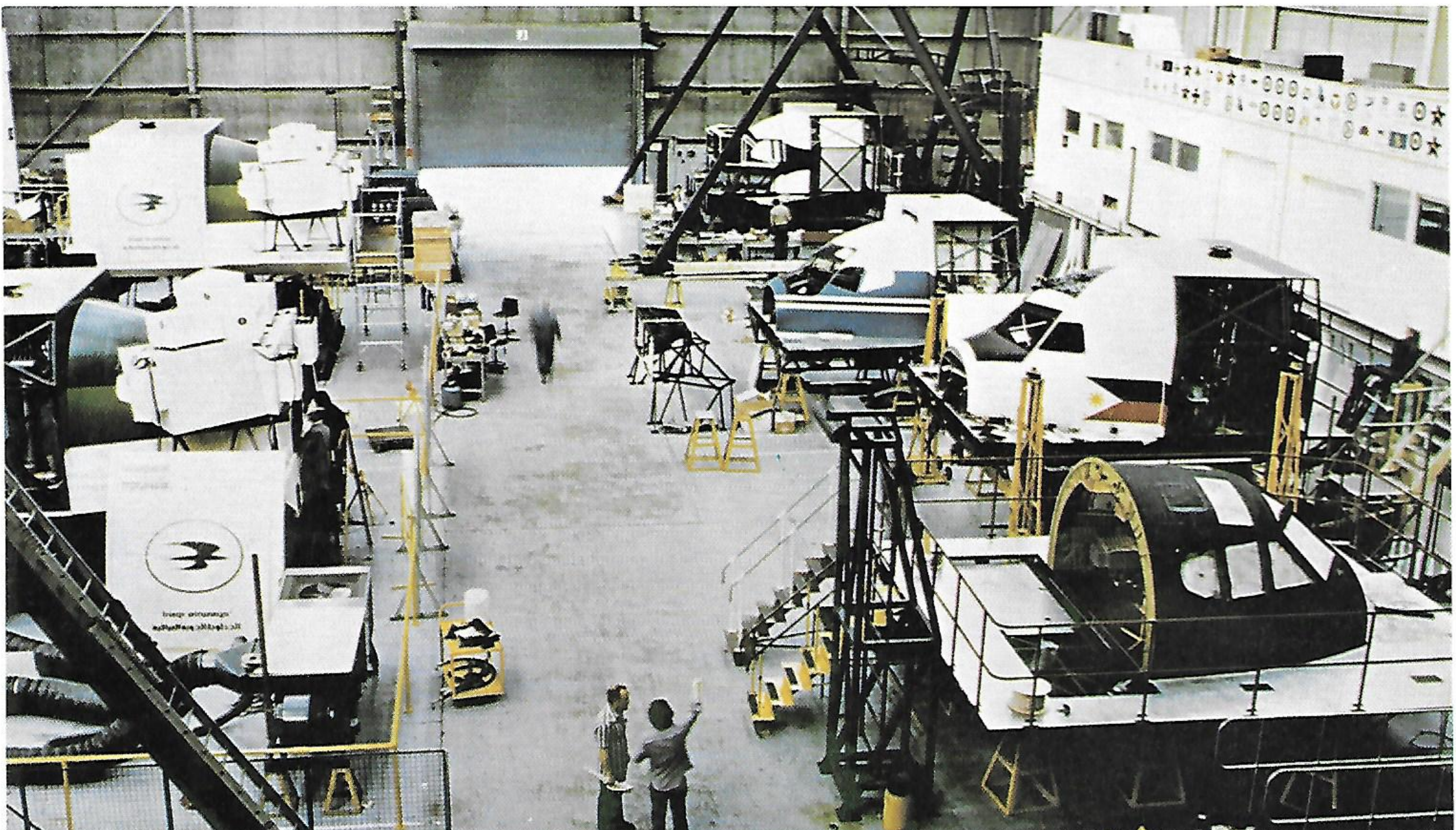
Partial view of the Main Shop with flight simulators being built for various airlines. Redifon Simulation exports 80% of its production.
