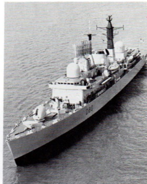
Armed with the Sea Dart Surface-to-Air missile, the HMS Sheffield also carries one 4.5 inch gun and a Lynx helicopter.
