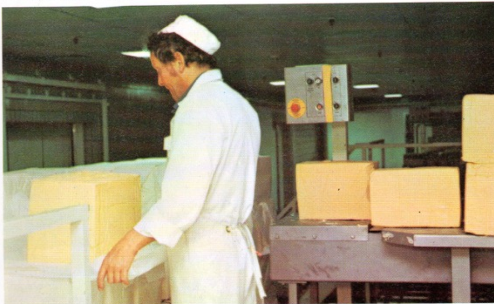
After conditioning, which takes about 56 hours, the butter is conveyed to the stripping aisle where the parchment is removed. This is the only occasion during processing that butter is exposed to air and the area is maintained in a pharmaceutically sterile state, with operators under strict hygiene constraints.
