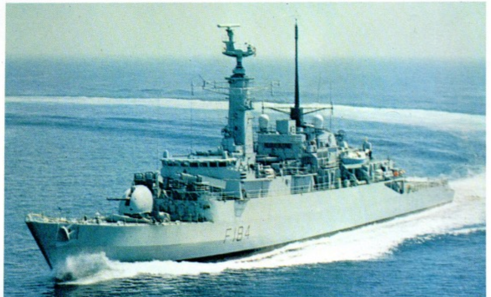
HMS Ardent, a Type 21 frigate, is one of a class of nine built between 1969 and 1978. She is armed with ship-to-ship missiles, anti-aircraft missiles, torpedoes and carries a Lynx helicopter. Her complement is 13 officers and 162 ratings.
