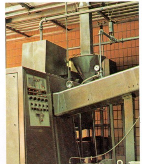
From the stripping aisle the butter enters the packing hall and is fed into this type of machine which re-works and softens the butter for packing and automatically standardises the moisture and salt content.
