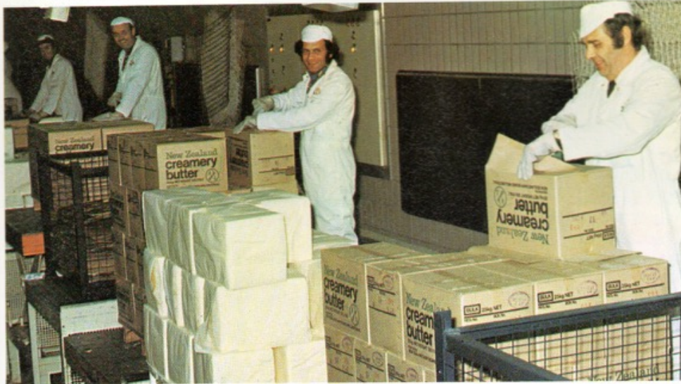
The first step before the packing operation begins is the "de-cartoning" of the butter when it is taken from cold storage.
