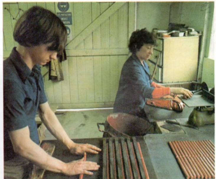
The wax is weighed, rolled and formed into the normal rectangular sticks ready for shipping.
