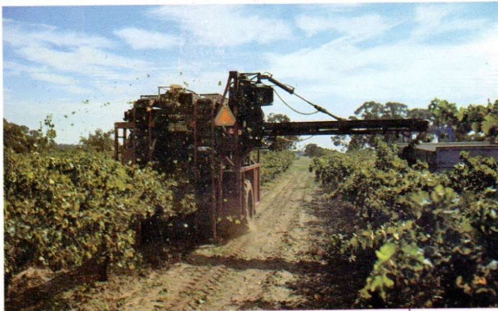
The vine leaves fly as a mechanical grape harvester picks some of the crop in the 1980 Australian vintage. Nearly three-quarters of Australian vine-grapes are now harvested by machines.
