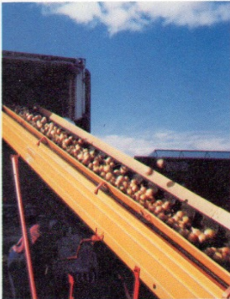
The bulk onions are loaded by a conveyor belt with an adjustable head which carries them directly into the container.
