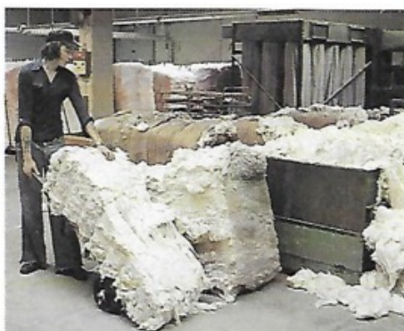
Before the manufacturing process begins, the cotton bale is broken open (left) and allowed to expand from its compressed state. Then bales of different cotton lots (right) are blended to obtain the required strength and quality in the finished thread.
