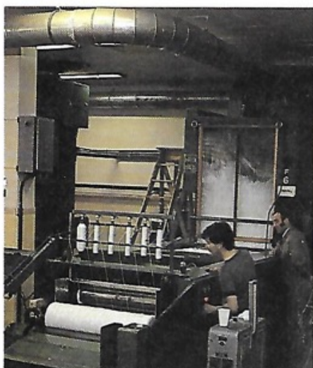
Then cotton is then fed into the machine in the photograph where after blending and scutching, it emerges fleece-like in the form of a lap.
