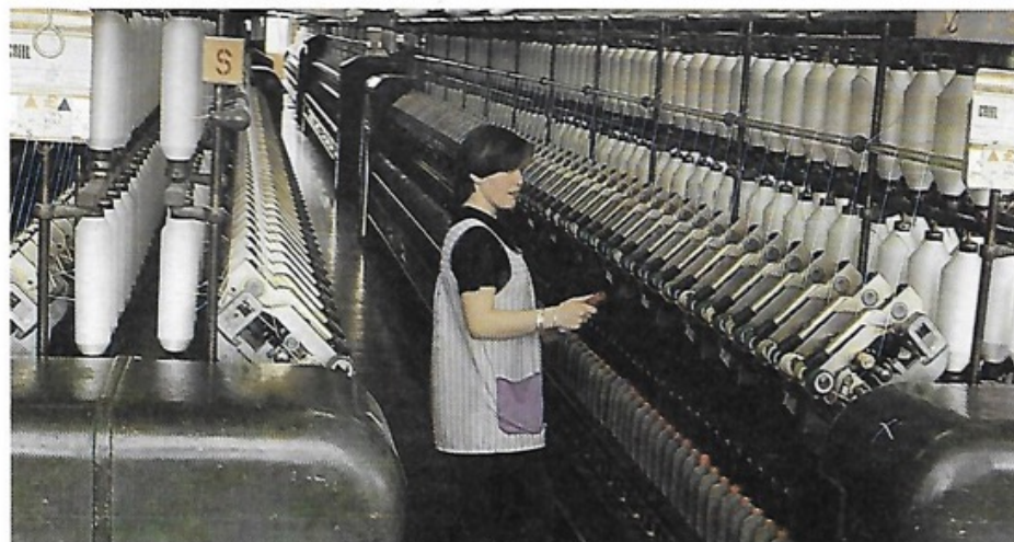
Synthetic staple polyester being ring spun at the Ferguslie Mill. Automation means that fewer employees are needed to process the thread but Coats still have thousands of workers, many of whom have spent their lives with the company.
