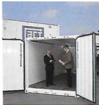
The recycling of 1,250 refrigerated ACT containers to improve thermal efficiency is taking place at Concargo's plant at Weston-super-Mare. The containers are stripped down completely and then rebuilt. In the photographs (left to right) the flooring rails are laid; polyurethane foam for insulation is press-injected in panels; the components are riveted; the inspection of newly recycled container is carried out by Mr. Bernard Glynn (left), ACT Services' Container and Equipment Inspector in charge of approving the completed work, and Mr. Alan Hollier, Estimator, of Concargo.
