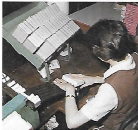
Thread coming off the production line and being packaged. Coats' threads are produced in three main finishes — soft, glacé and mercerised.
