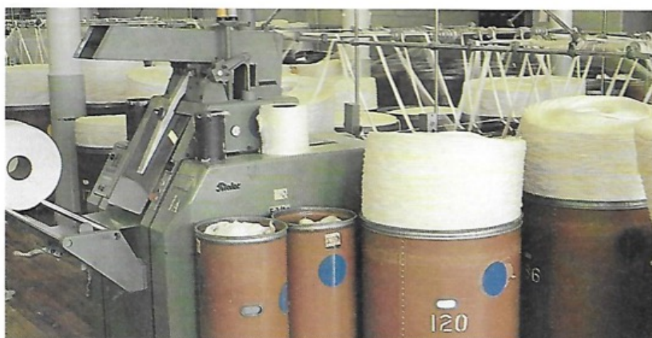
After carding, which converts the lap into the form of a soft rope or sliver and begins to lay the cotton fibres parallel to one another, several slivers are combined, extended in length and reduced in diameter (in this photograph). More and more impurities are removed by each process.
