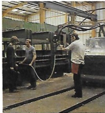
The recycling of 1,250 refrigerated ACT containers to improve thermal efficiency is taking place at Concargo's plant at Weston-super-Mare. The containers are stripped down completely and then rebuilt. In the photographs (left to right) the flooring rails are laid; polyurethane foam for insulation is press-injected in panels; the components are riveted; the inspection of newly recycled container is carried out by Mr. Bernard Glynn (left), ACT Services' Container and Equipment Inspector in charge of approving the completed work, and Mr. Alan Hollier, Estimator, of Concargo.
