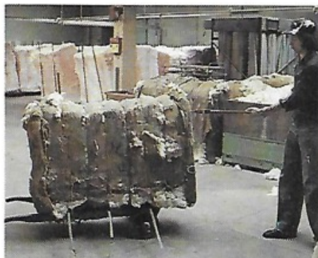
Before the manufacturing process begins, the cotton bale is broken open (left) and allowed to expand from its compressed state. Then bales of different cotton lots (right) are blended to obtain the required strength and quality in the finished thread.
