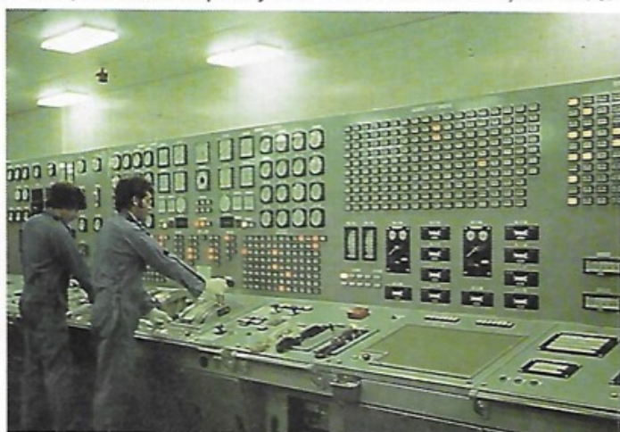
A view of the engine room (left) of the "City of Edinburgh" showing the newly installed 25,690 horsepower, 7-cylinder diesel engines, which give a service speed of 23 knots. The sophisticated control panels (right) monitor the smooth functioning of the engine room 24 hours a day.
