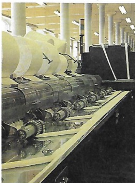
During combing, rapidly rotating needles thoroughly comb the lap from end to end and unwanted short fibres are removed. This ensures the sliver leaving the combing machine consists only of the longer cotton fibres.
