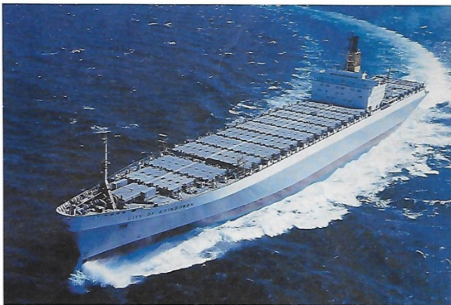
BLC's "City of Edinburgh" completing trials following her conversion from steam to diesel. At the same time, container capacity was increased to over 3,000 TEUs.
