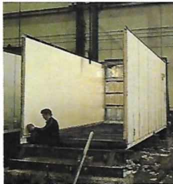
The recycling of 1,250 refrigerated ACT containers to improve thermal efficiency is taking place at Concargo's plant at Weston-super-Mare. The containers are stripped down completely and then rebuilt. In the photographs (left to right) the flooring rails are laid; polyurethane foam for insulation is press-injected in panels; the components are riveted; the inspection of newly recycled container is carried out by Mr. Bernard Glynn (left), ACT Services' Container and Equipment Inspector in charge of approving the completed work, and Mr. Alan Hollier, Estimator, of Concargo.
