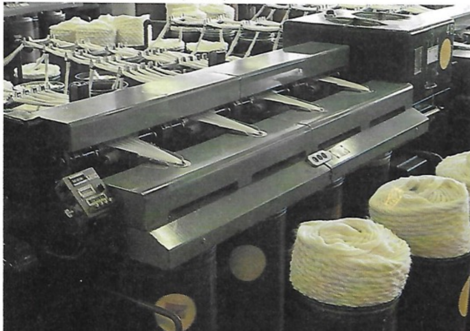
Slivers are fed into high speed frames which reduce each sliver from a diameter of about one inch to a thickness rather less than that of a pencil. The cotton is now termed "roving" and then the roving goes through spinning, during which it is again drawn out and reduced in diameter. The single yarns produced by spinning are not nearly strong enough for sewing and two or more yarns must be combined to make a thread.
