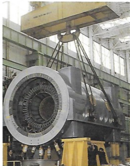
Stator frame for Castle Peak Project is carefully lowered into position for tests to be carried out. Even inside the plant, it takes a tremendous amount of expertise to shift these giant pieces of equipment.
