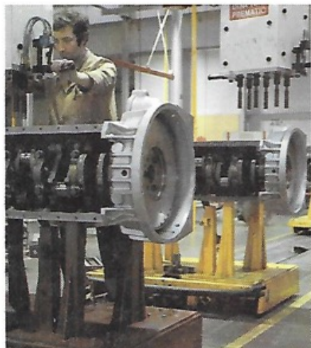
Long Block Stage, where the standard Cummins engine begins to be built up using the latest technology.
