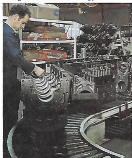
Laying in the bearing shells at the start of the engine assembly at Cummins' plant at Shotts.
