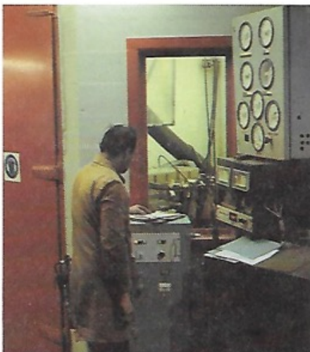
Extensive tests are carried out on the new 10-litre engine in an Engineering Test Cell.
