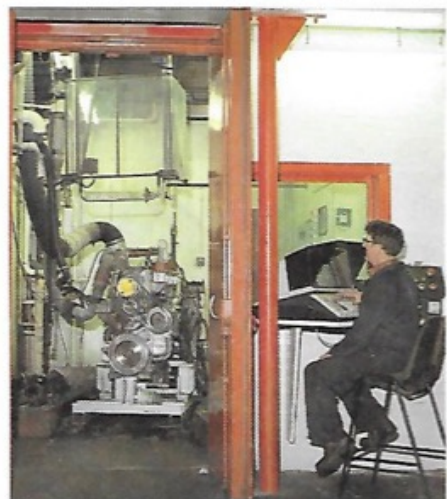
Production Test Cell, where every completed engine gets tested under computer control.
