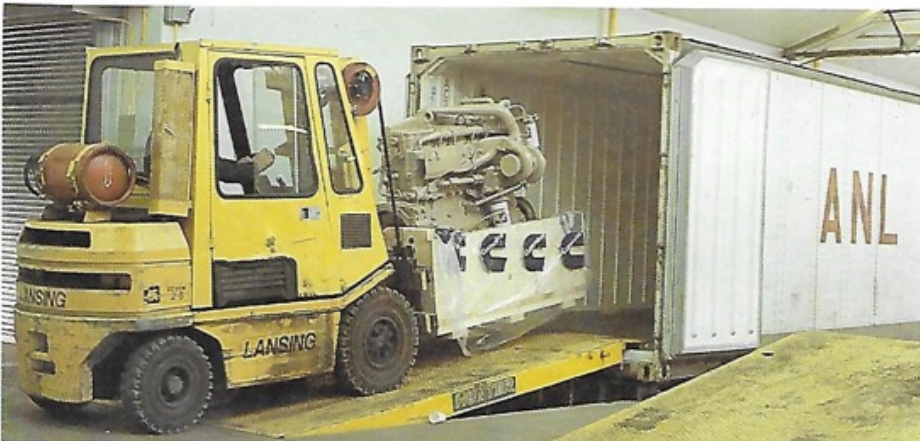
An engine is carefully loaded into a container to be transported to the docks. A 20-foot insulated container can carry six of these engines.
