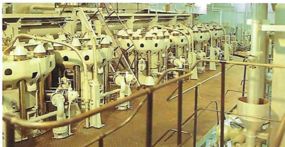
...With her new MAN diesels giving a service speed of 23 knots and each motor providing 25,690 horsepower.
