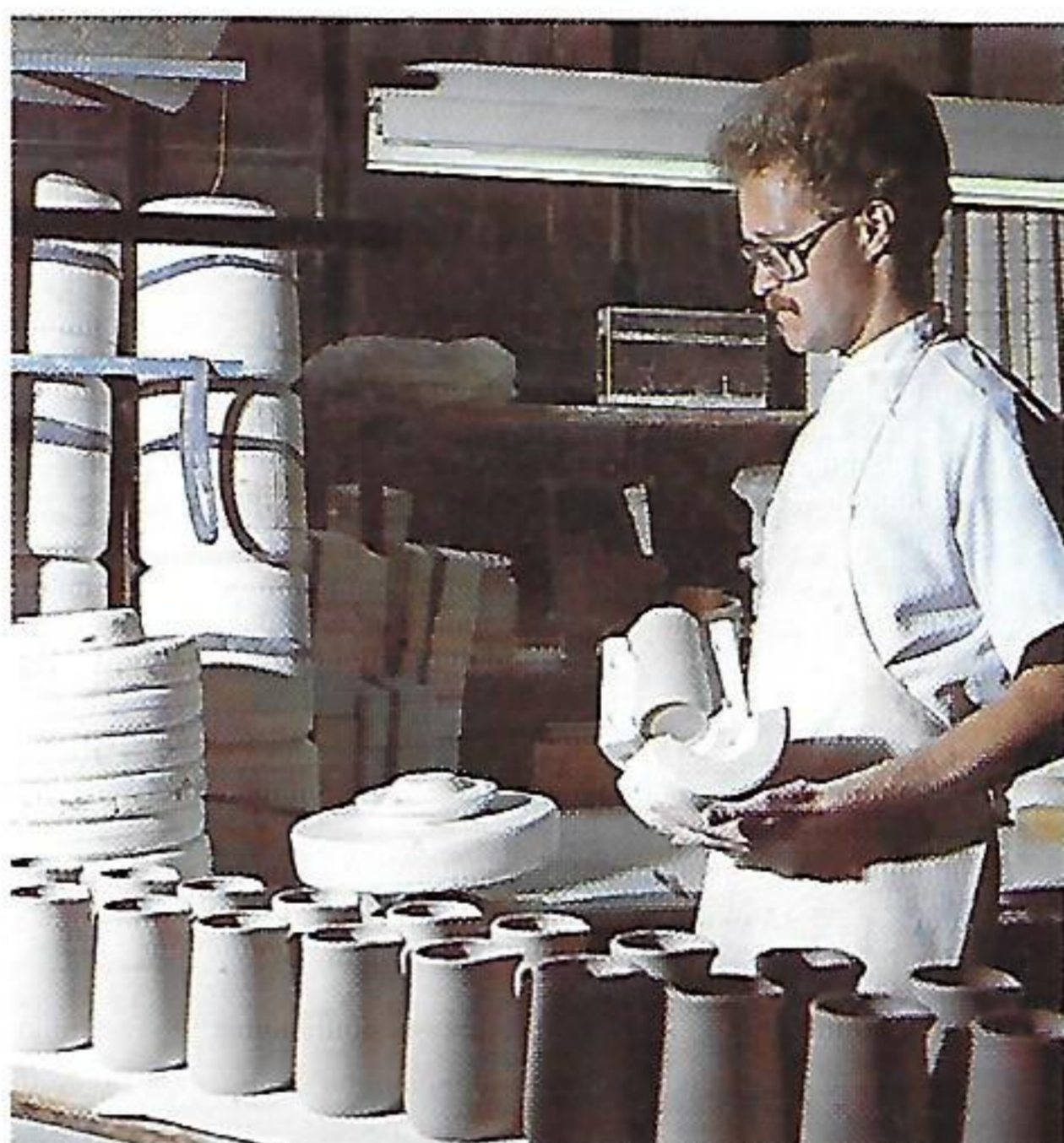
Opening moulds. Liquid clay "slip" goes into a plaster mould, then excess slip is poured off.
