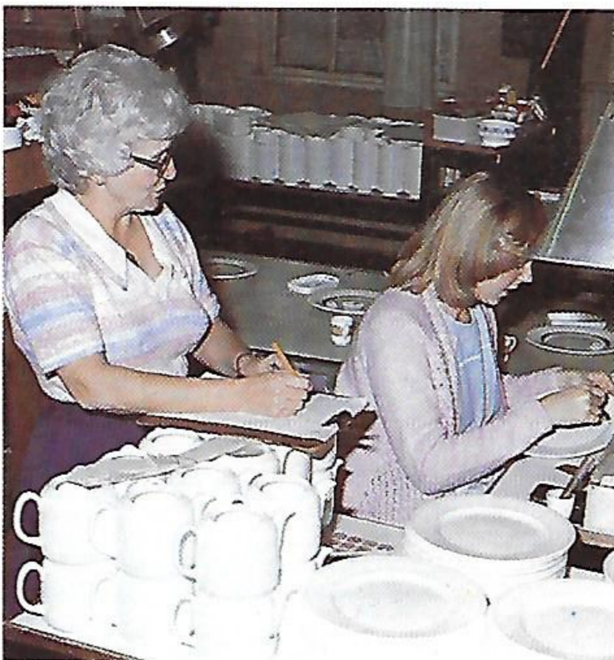
Application of multi-colour transfers. Constant checks are carried out at every step of production.
