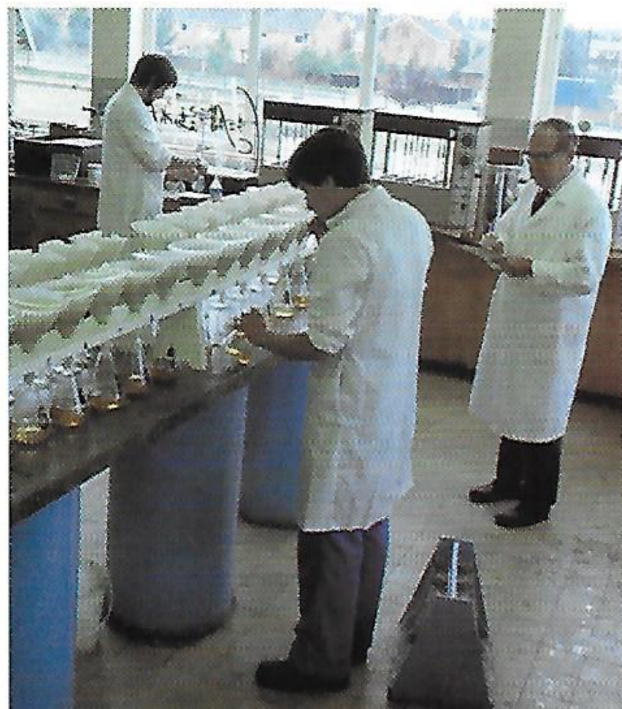
In the laboratory at ABM's Wallingford Plant, Chief Chemist D. Ensor (right) checks on samples of wort being taken for testing for total soluble nitrogen (tsn) while another member of staff carries out a filtration (background).
