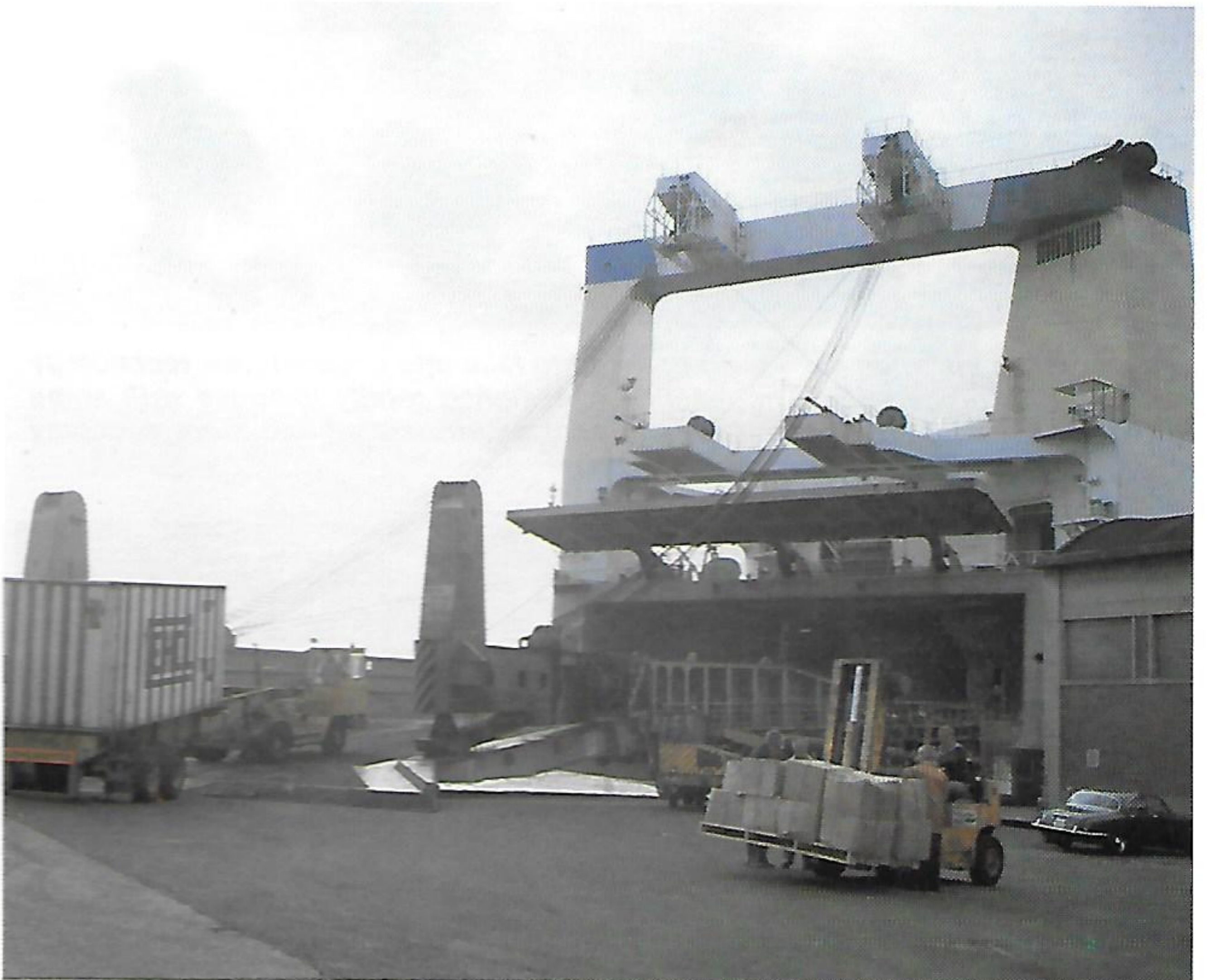
An EHCL container starting up the 12-metre-wide ramp of the "Kolsnaren" during loading at Tilbury on the new ro-ro service direct from the U.K. to Namibia, South Africa and Mozambique. The vessel offers a comprehensive and flexible capacity for cargo mix which includes 673 TEUs on the upper deck, a clear height of 6.7 metres at entrance deck with 3.1 metres in the lower decks and two bulk liquid tanks with 713 cbm combined capacity. Also, dedicated car decks for 125 cars, two refrigerated chambers of 3700 cbm/2000 cbm, plug-in reefer points and a limited number of clip-on units.
