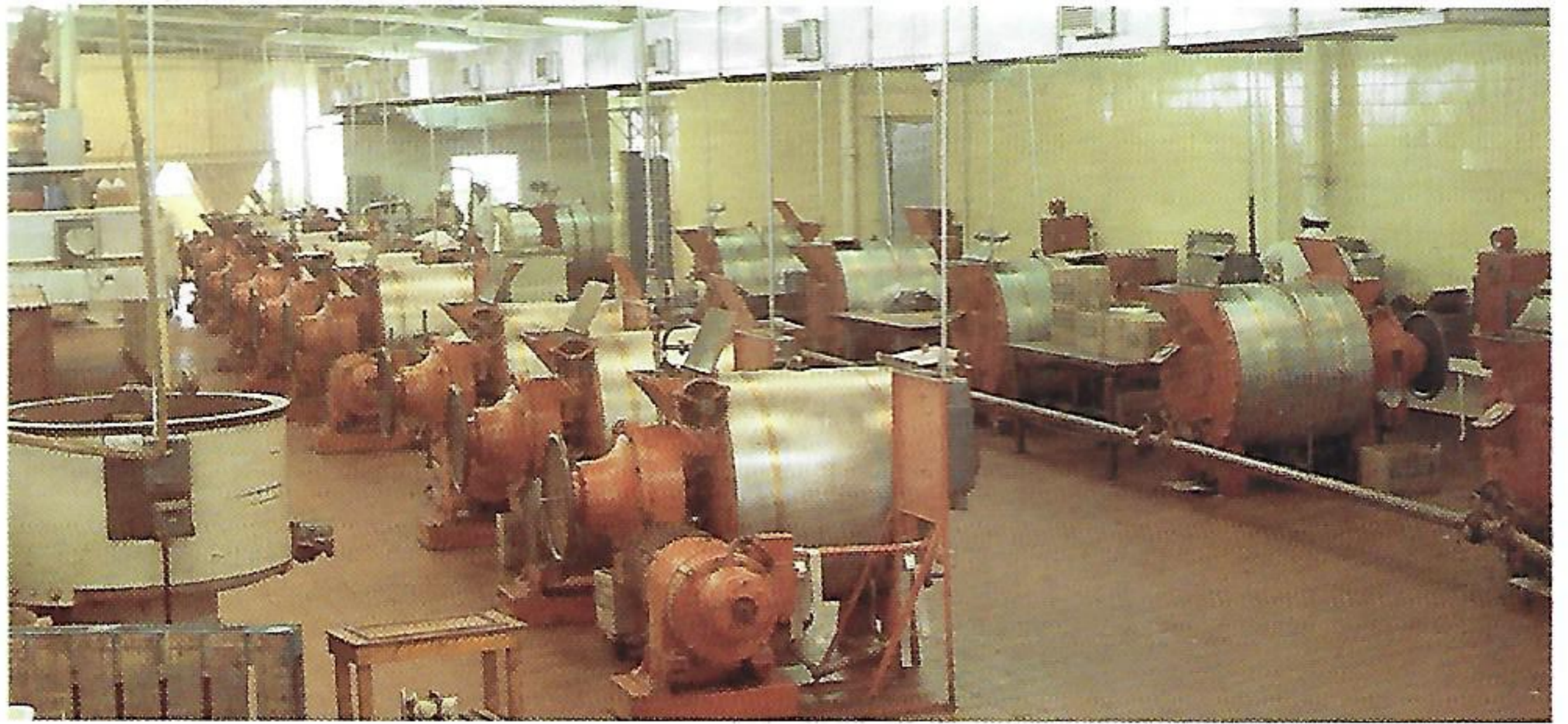
Partial view of the chocolate refining section. Tunnock's produces 12 tonnes of caramel and ten tonnes of chocolate each day and they are proud that only the finest ingredients are used.
