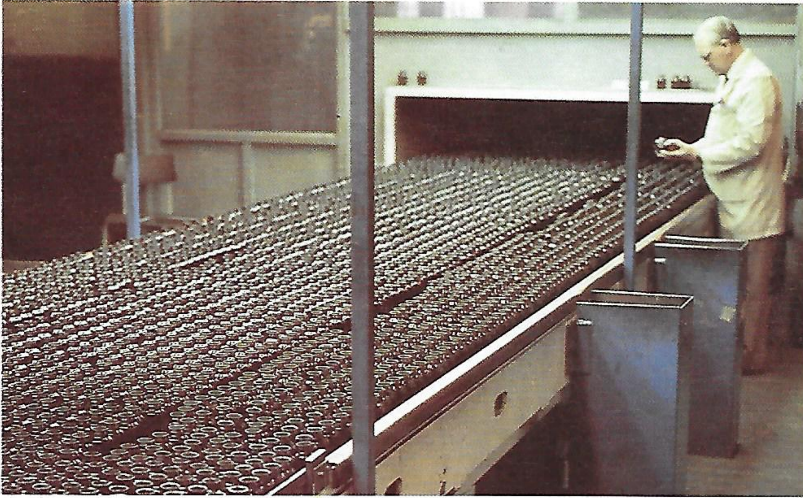
LOTTA BOTTLE! — Pictured is the first stage of the inspection process at the Rotherham Works where up to one million glass containers are produced each day.
