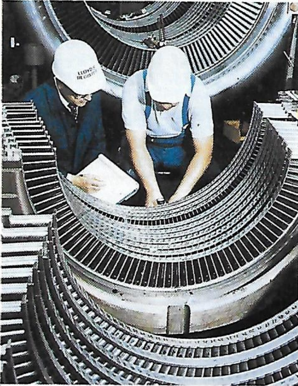
Industrial inspection forms an important part of LR's activities. In the photograph, an LR surveyor (left) supervises measurement of turbine equipment for an Australian power station.
