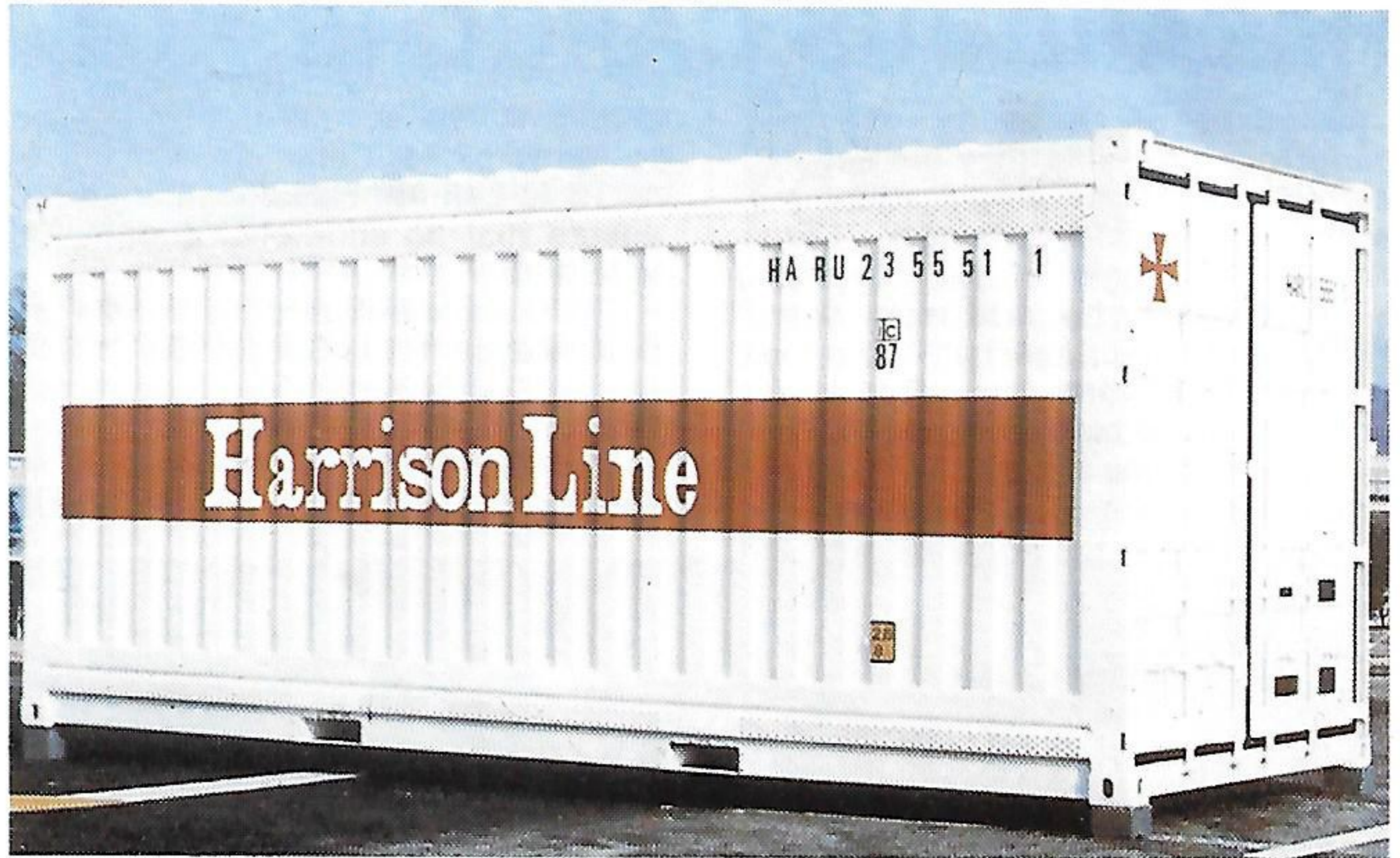
A ventilated container belonging to Harrison Line which is used in shipping coffee. Air inlet baffles can be seen at the base of the side wall. Harrison Line was one of the pioneers of this method of shipping coffee.
