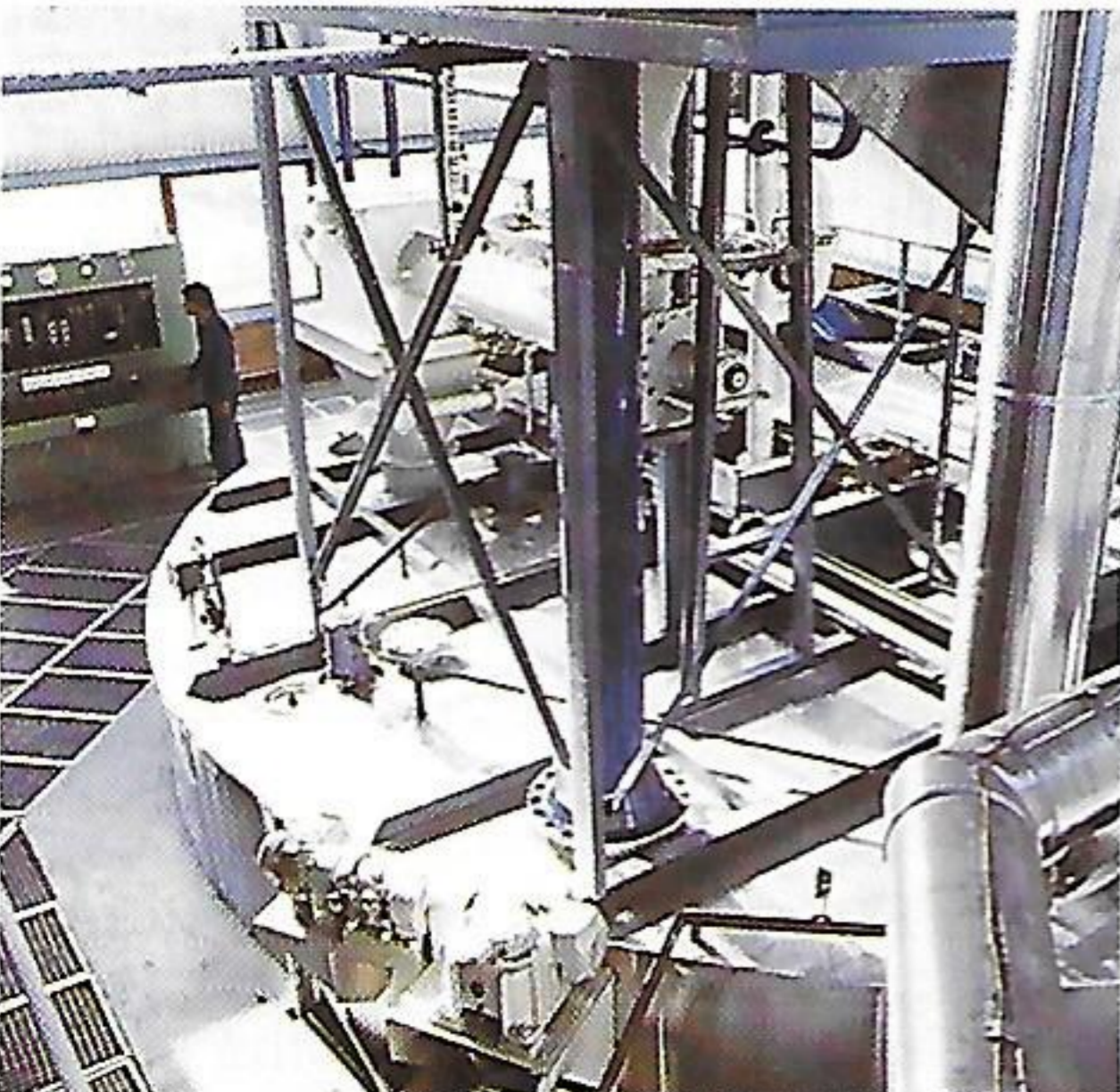
The traditional continuous rotary extractors manufactured by Simon-Rosedowns, like the one pictured, are still available for specific duties.
