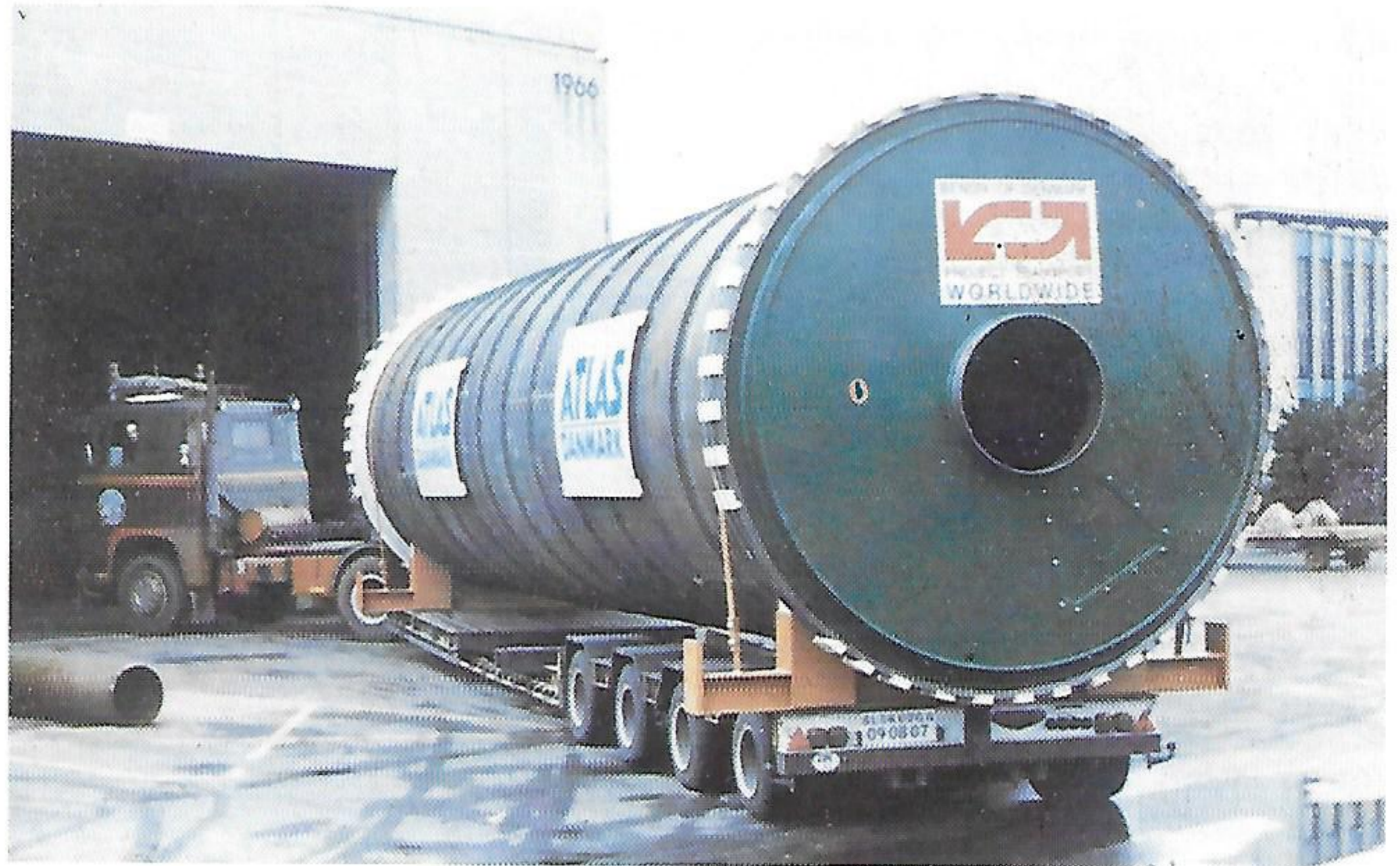
This giant drum for a RUDD 100 plant is ready to leave the Atlas-Danmark factory for its long journey to Bangkok. Weighing 20,000 kilogrammes, the drum will form part of a plant to be used for drying sugar-cane tops to provide material for livestock consumption.
