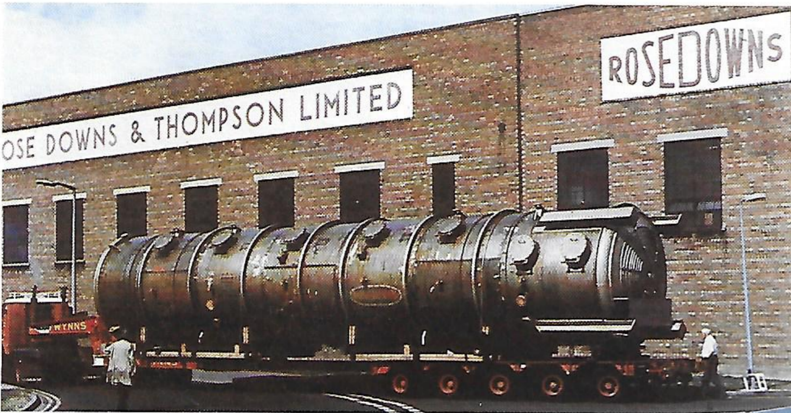
This 30,000 lbs per hour Rosedowns-Votator Semi-Continuous Deodoriser — the largest ever shipped from the Hull factory — was photographed as it was ready to leave the works for Tilbury's Northfleet Hope Terminal bound for PTL Margarine in Murarrie, Australia.
