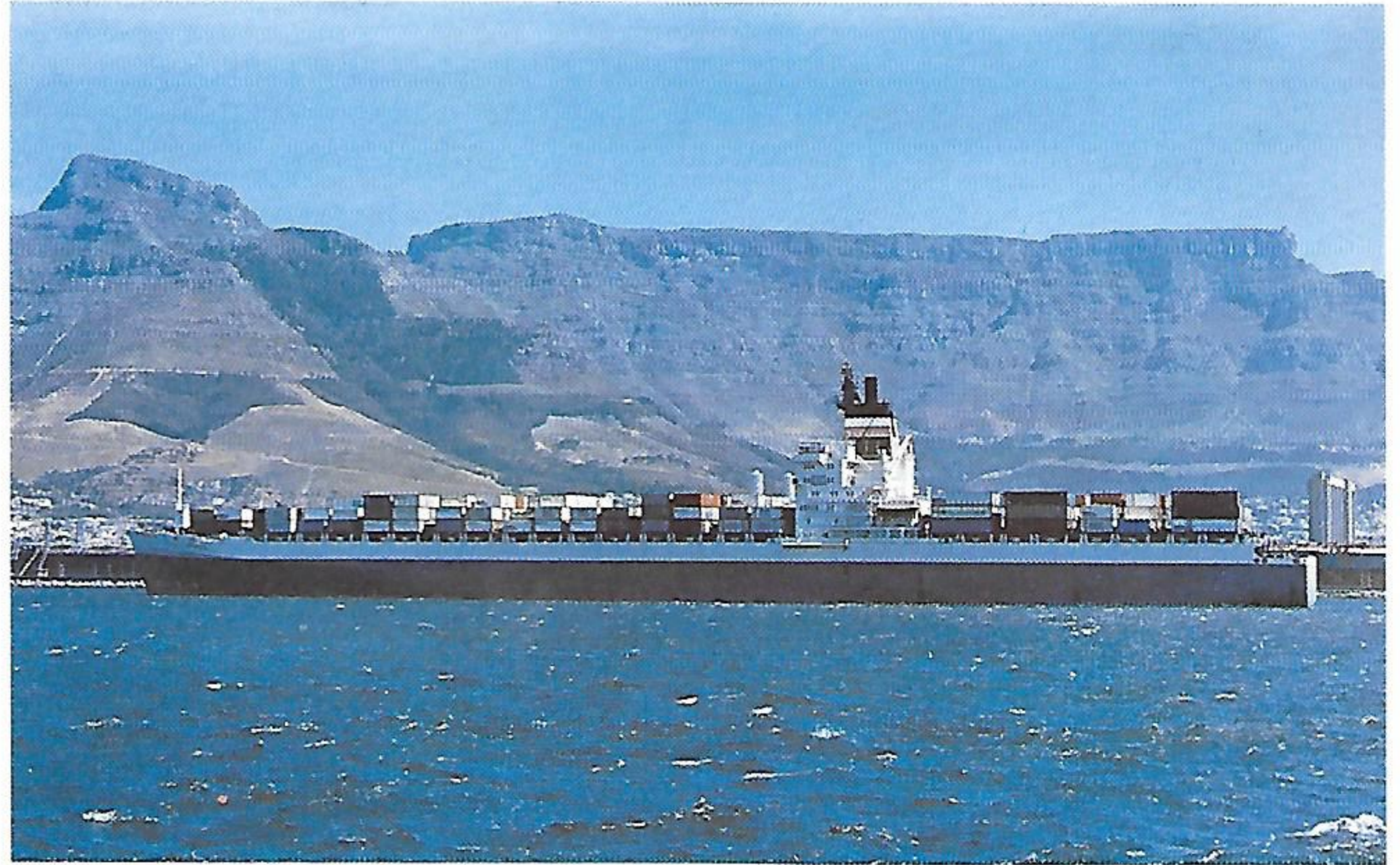
EHCL's modern containership "City of Durban" is an example of some of the major developments that have taken place over the past century on the Europe/South Africa route. The highly efficient "City of Durban" has a capacity of 2,400 TEU's and a cruising speed of 21.5 knots.
