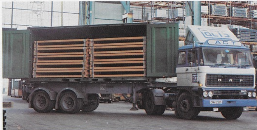
Long pieces of shelving are loaded easily into the side-door containers used by C.A.M.E.L. for the shipment.
