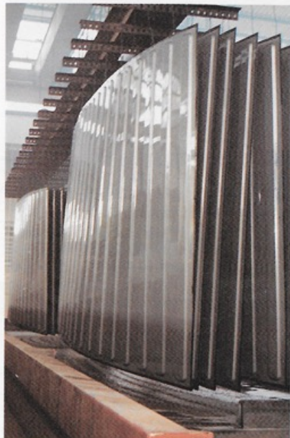
After the galvanising process is complete, the roof panels and sidewalls are passed through a passivation bath.
