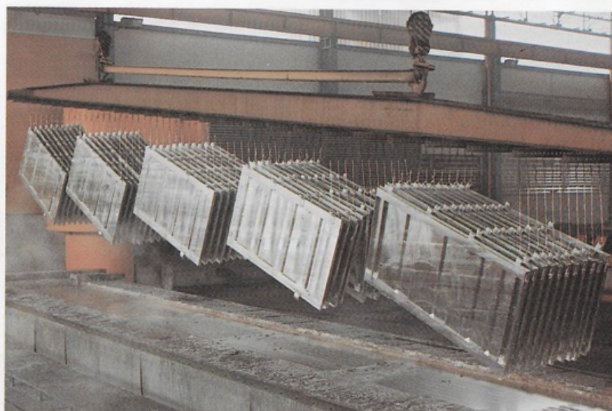
All sub-assemblies are individually suspended to ensure that there is no contact which could prevent the formation of the zinc layer in the manufacture of BLC's galvanised containers.
