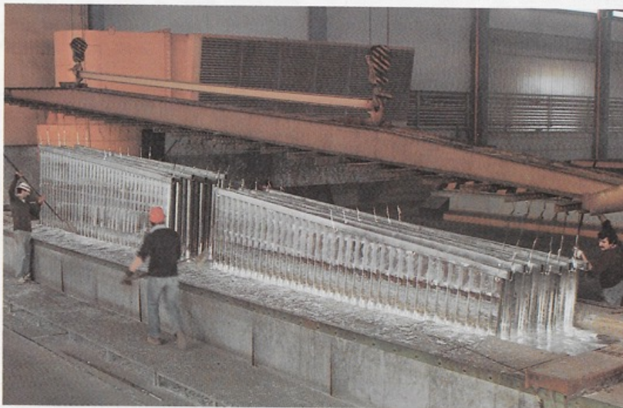
Zinc baths at the galvanising plant used by Officine Franchin are 3.5 metres deep and large enough to accommodate 20-foot and 40-foot sidewalls without double dipping.
