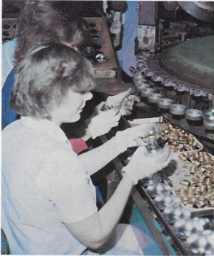
Reflector lamp in the final process of capping.
