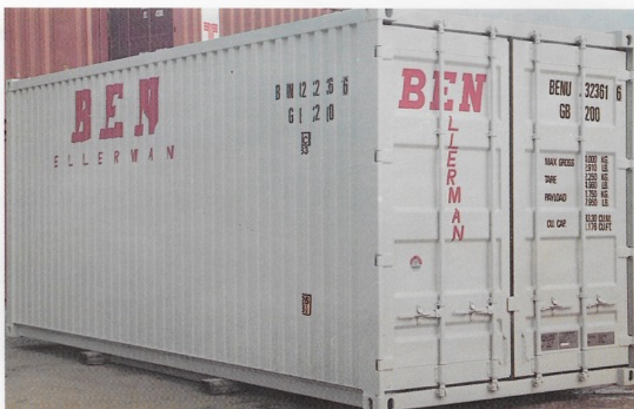
One of the latest Ben Line galvanised steel dry freight boxes, part of an order of one thousand for this particular type of container, which has been manufactured by Officine Franchin of Italy.
