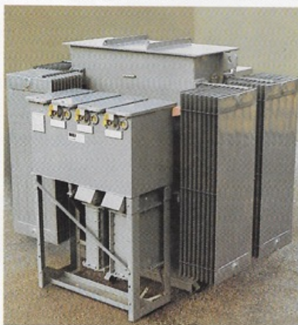
Pictured is a 1000kVA package sub-station using a sealed transformer and having HV and LV switchgear on opposite sides of the unit for compactness. This is one of a wide variety of transformers manufactured by Peebles Distribution Transformers.
