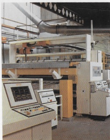
Two of the sophisticated pieces of machinery being supplied for the corrugated cardboard box-making factory at Riyadh are a Simon 250 Split Line Slitter Scorer (left) and a Simon 300 VSF Single Facer (right).
