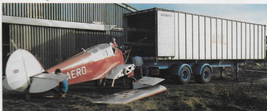
Final preparations are made for the aircraft to be stowed in the container after its wings, etc. have been removed.
