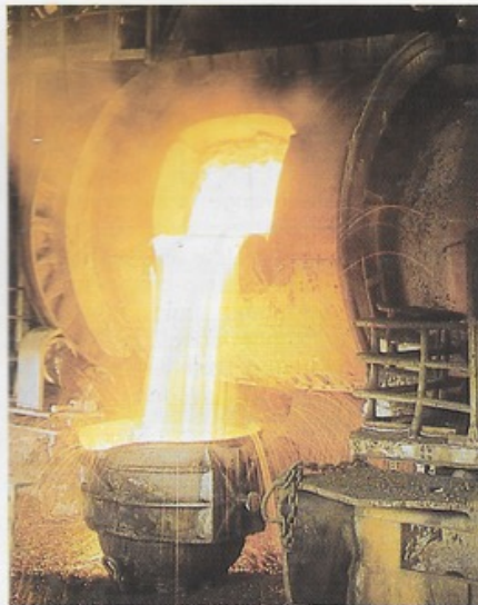
Long hose drilling (left) is one of the methods used in mining copper in Zambia. Tapping slag converter furnace (centre) – part of copper processing. Anode Casting Wheel (right) at Luanshya Mine.
