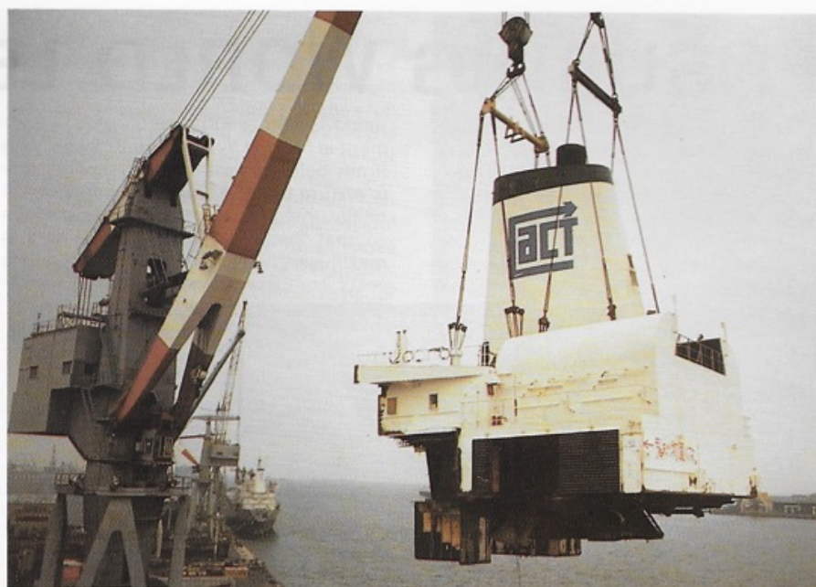
Funnel being taken off one of the ACT ships as work begins on the re-engining and refurbishment to bring it into the 1990s.
