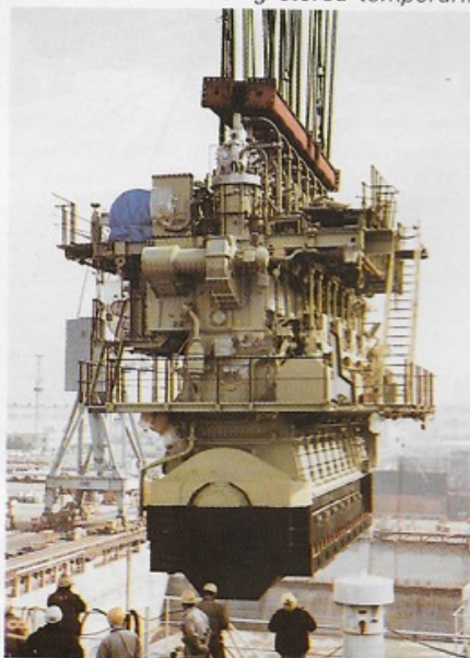
One of the main diesel engines being installed in the ACT Ships - an IHI/Sulzer 8RTA62 type.
