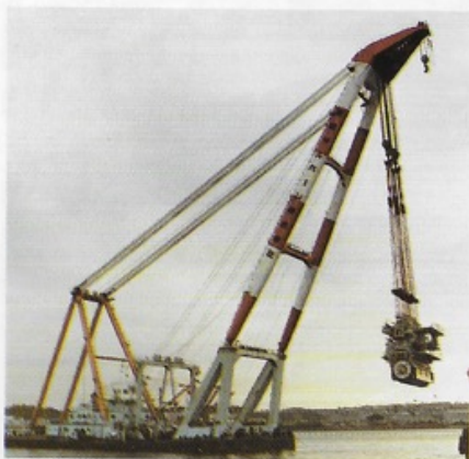
A new main engine being taken out to the ship by a giant floating crane.
