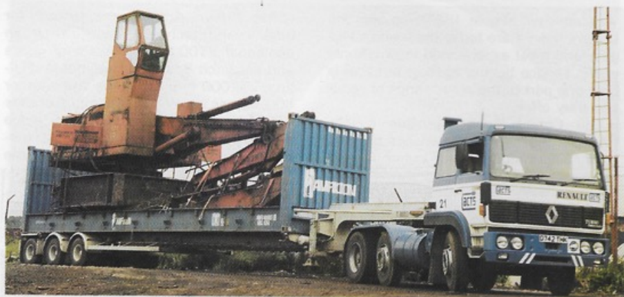
One of the cranes had to be moved across the yard to the quay and was lifted onto a low-loader supplied by ACT Services.
