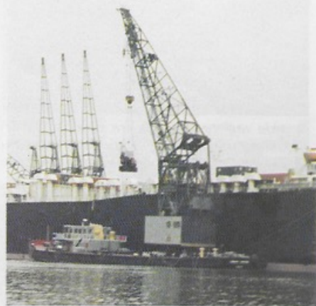
Tilbury's floating crane, "London Samson", manoeuvres the cranes for loading aboard ship.
