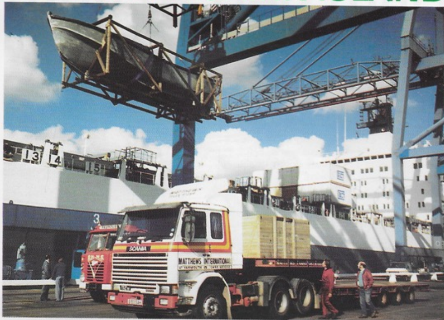
The motorised aluminium longboat is loaded aboard the "ACT 8" at Tilbury's Northfleet Hope by the Dock's gantry crane, to be securely fixed on deck for the long voyage.
