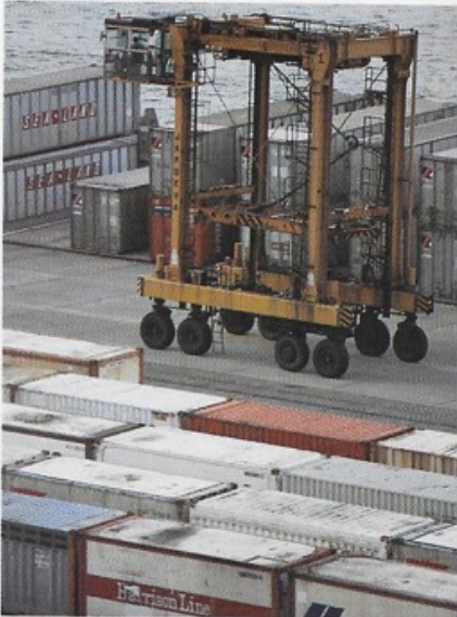
Three-high Straddle Carrier at work in the Puerto Limon Container Terminal, which is equipped with the most up-to-date equipment.
