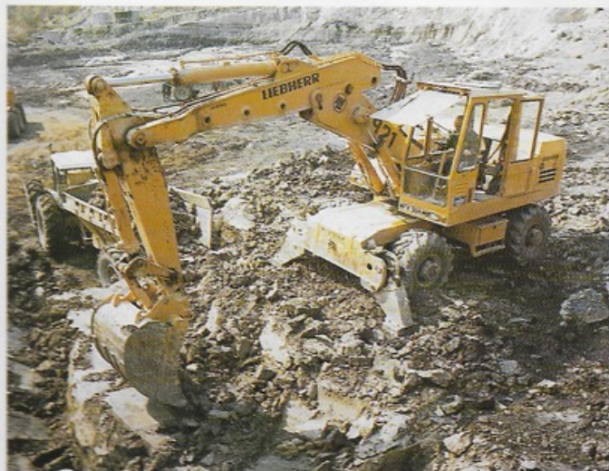
The photograph at left shows open-cast extraction of ball clay at Meeth, in North Devon. Some of the highest quality china clay in the world is to be found in South-West England. The picture at right shows a ball clay store and the grey-brown colour of the material in its raw state. When it is fired, however, it becomes ivory in colour.
