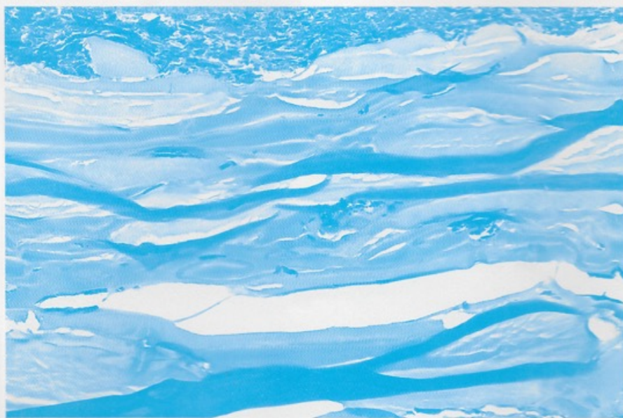
Much of the world's production of china clay today is used in the paper industry. The photograph shows a cross-section of a printed paper sheet lightly coated with china clay and magnified 1,600 times.
