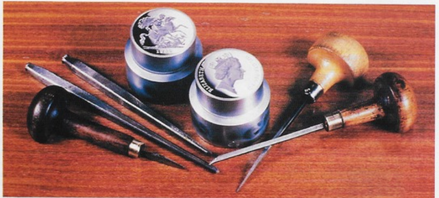
A pair of dies, produced in relief from an electrotype copy of an artist's plaster model, and some hand tools. Since the beginning of this century hand-engraving of original coinage dies has been largely superseded by the use of the reducing machine.
