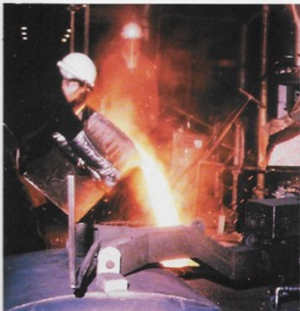
Melting, rolling and blanking is carried out in the Furnace Area where temperatures of 750 degrees Centigrade for bronze and 900 degrees Centigrade for cupro nickel are reached.
