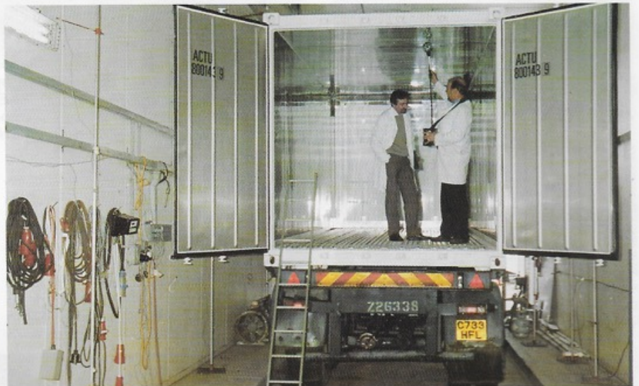
In the photograph above Jim Mansfield (right) of the Shipowners Refrigerated Cargo Research Association (SRCRA), and Bob Banks, Refrigeration Engineer, of ACT Services, measure air speed in one of the new containers in a test chamber at SRCRA, while in the photo below Jim Mansfield checks a print-out of thermal test data.
