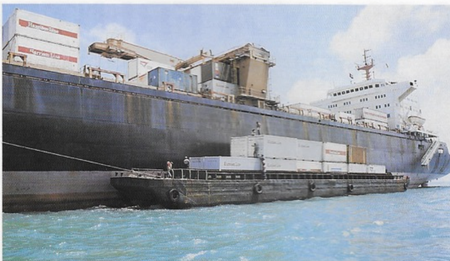
Containers being unloaded by deck gantry crane onto barges at Belize, carrying equipment for the new Kier airport contract. Belize is a lighter port and ships anchor 4½ miles offshore.
